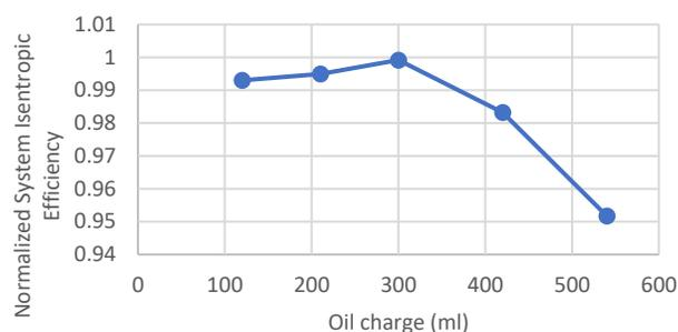
**Figure 4:** Normalized weighted average system isentropic efficiency in dependence on the oil charge.
