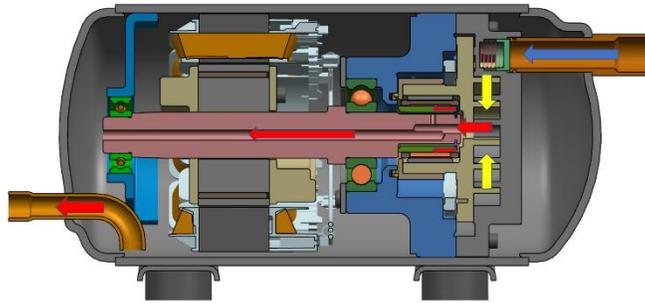
**Figure 2:** Sump-less compressor with discharge port in the orbit scroll
