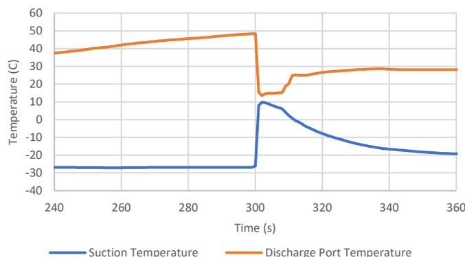
**Figure 3:** Suction gas temperature and temperature of the gas next to the discharge port.
