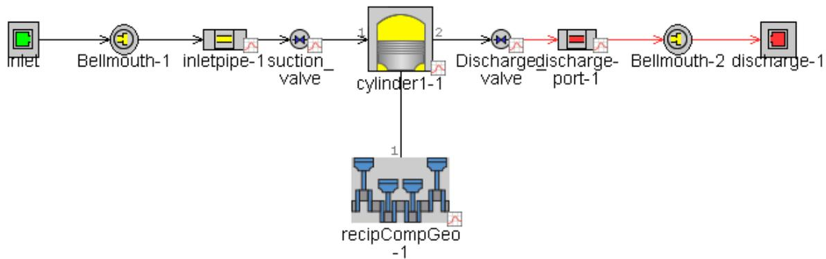
**Figure 2:** Schematic of compressor model in GT-Suite™.
