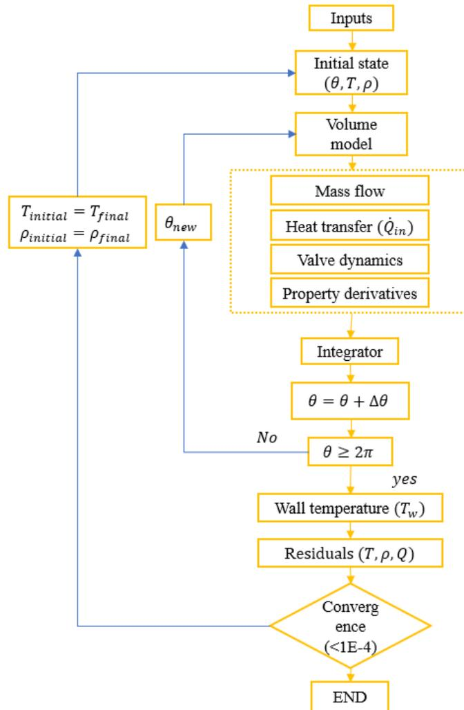
**Figure 1:** Flow chart for mechanistic chamber model.
