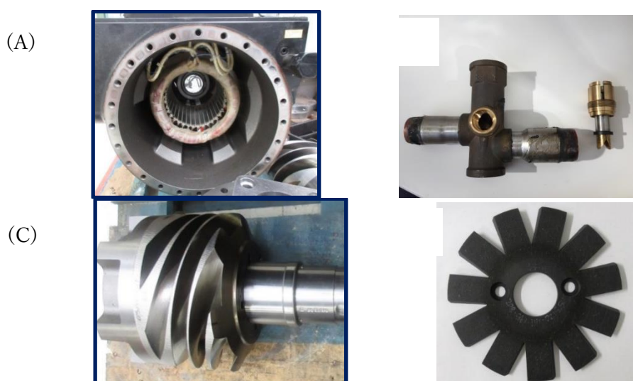
Figure 3: (A) Motor, (B) Expansion valve, (C) Screw rotor, (D) Gate rotor, after System Drop-in Test
