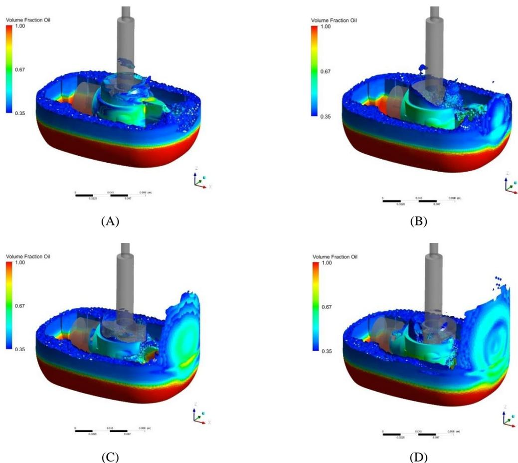
**Figure 5:** Oil volume fraction at (A) 270° of 3<sup>rd</sup> cycle (B) 180° of 7<sup>th</sup> cycle (C) 90° of 11<sup>th</sup> cycle and (D) end of 15<sup>th</sup> cycle
