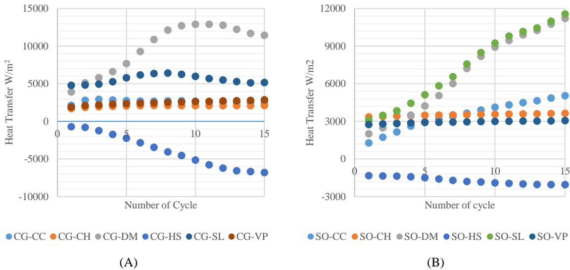
**Figure 6:** Cycle Averaged Heat transfer of various interfaces with (A) Cavity domain and (B) sump domain
