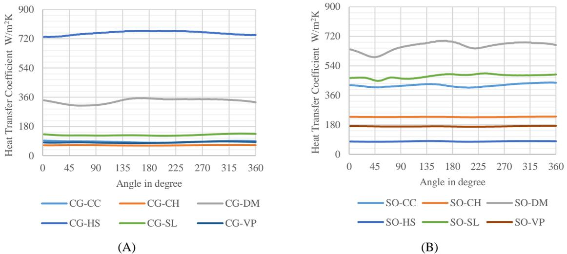
**Figure 7:** Variation of Heat Transfer Coefficients in a cycle of various interfaces with (A) Cavity domain and (B) Sump domain
