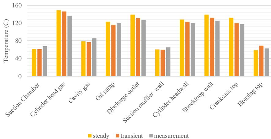
**Figure 8:** Comparison chart of temperature from 1D simulation
