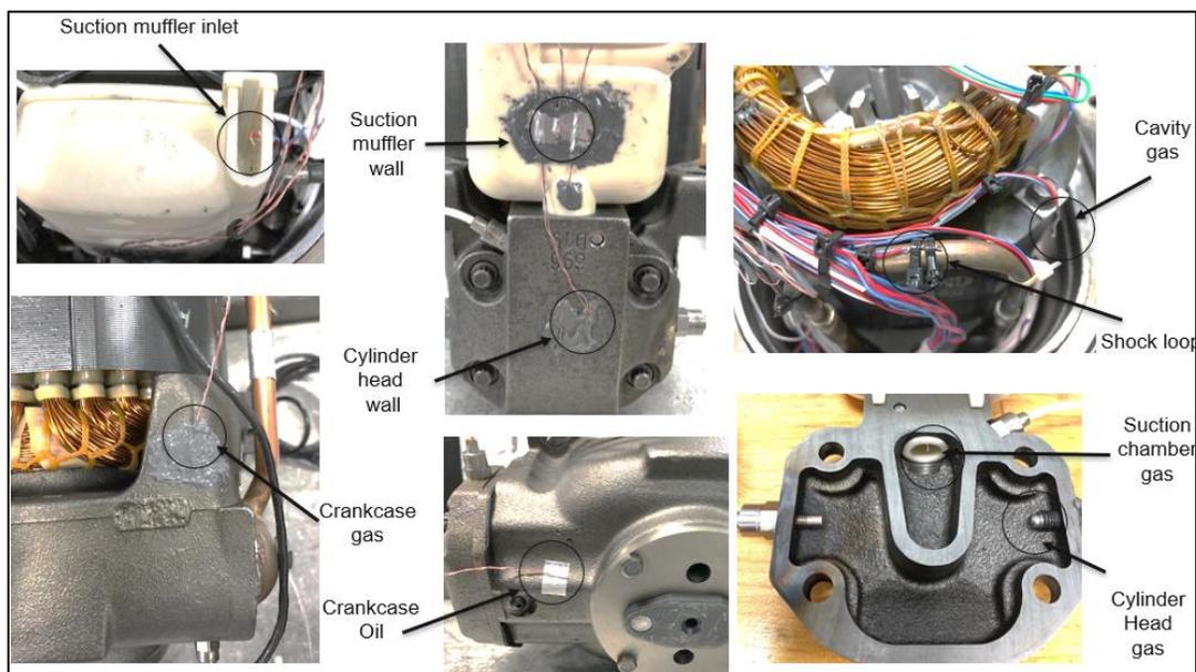
**Figure 3:** Thermocouples position - Compressor kit
