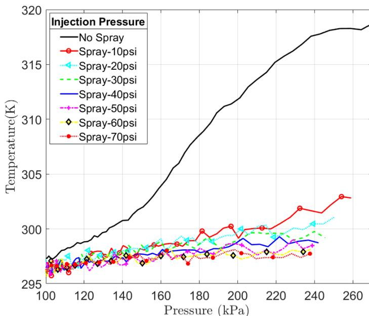
**Figure 5:** Temperature-pressure plot during compression
