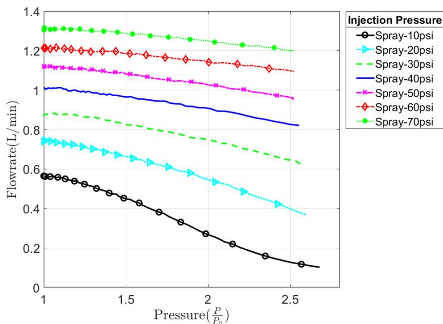
**Figure 6:** Flowrate of spray water for different injection pressures during compression
