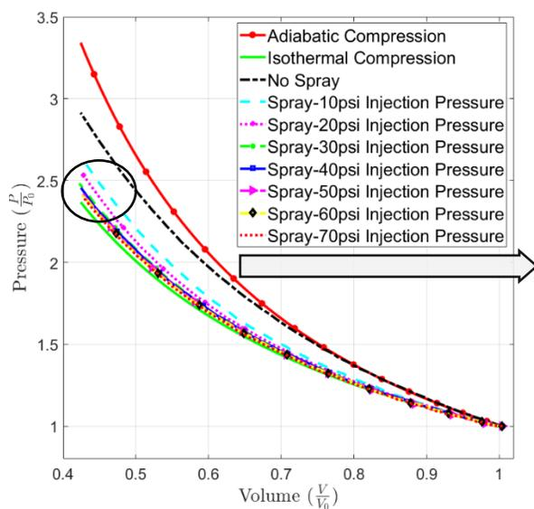
Figure 3: Pressure-volume during compression
