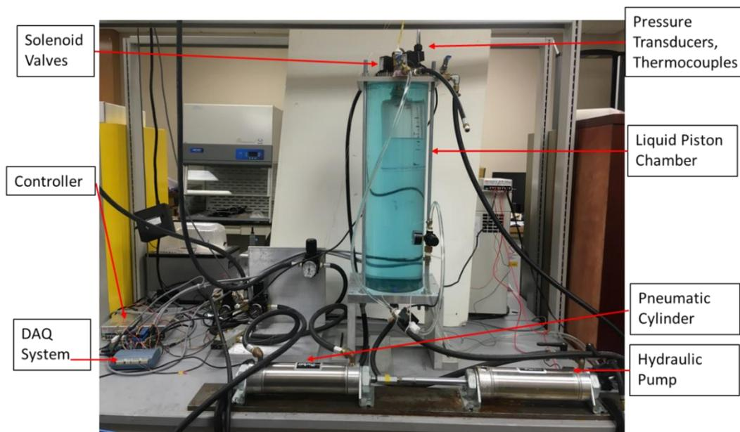
**Figure 1:** A table-top setup of Liquid piston compressor with spray cooling
