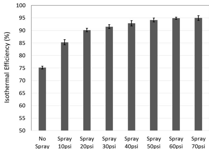
**Figure 7:** Isothermal Efficiency of Compression
