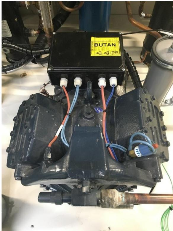
**Figure 2:** The prototype one-stage semi-hermetic 4 – cylinder piston compressor
