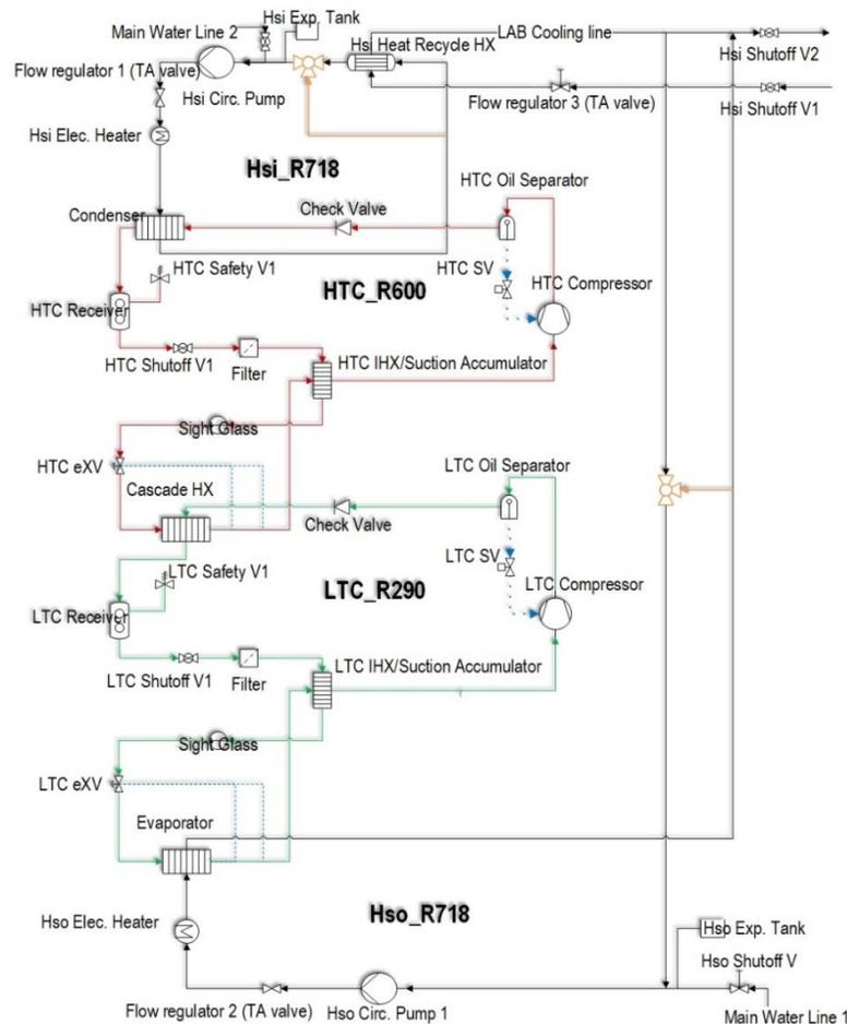
**Figure 1:** Schematics of the 20 kW cascade configuration heat pump with prototype butane compressor on the HTC
