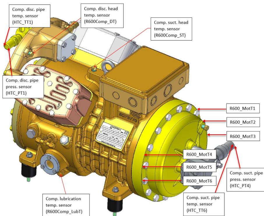
**Figure 3:** Pressure and temperature sensors distribution on the prototype compressor
