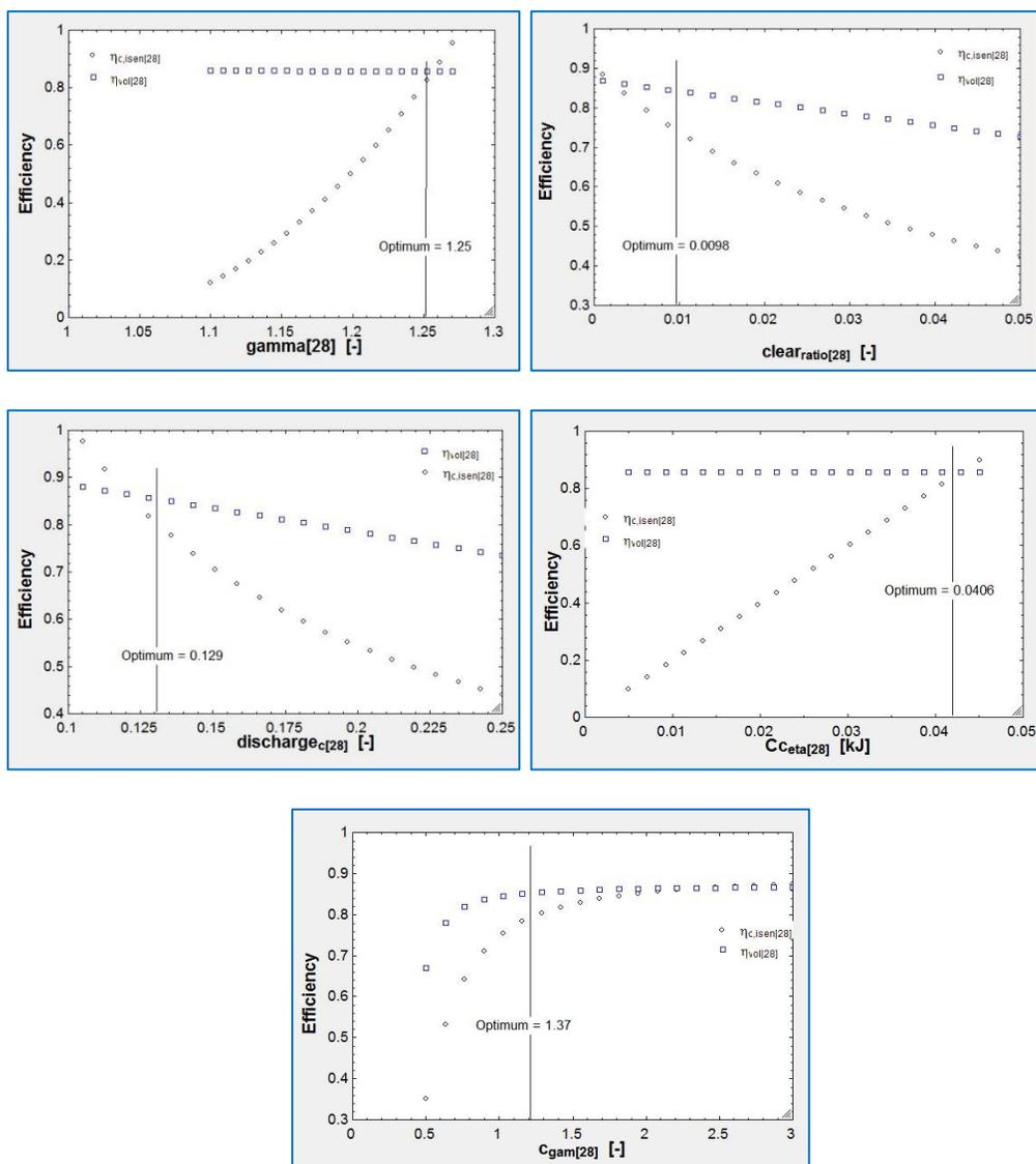
**Figure 9:** Above plots show the variation of isentropic  $\eta_{c,isen(28)}$  and volumetric efficiencies  $\eta_{vol(28)}$  with the primary design variables of the system. These parameters were optimized to achieve a low RMS error.
