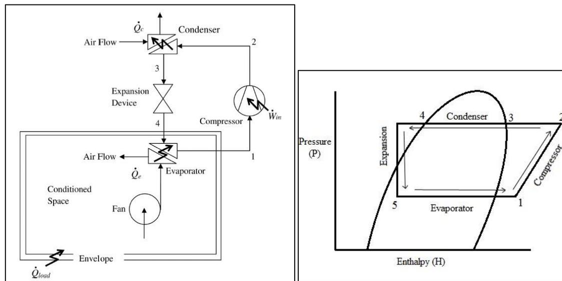
**Figure 1:** a) Schematic diagram of air conditioning cycle with all its components. Adapted from *Optimization of Cooling Systems* (p.4) by D.C. Zietlow, 2016 New York, NY: *Momentum Press Thermal Science and Energy Engineering Collection*. Copyright (2016) by Momentum Press. b) Property plot of pressure-enthalpy variations through different state points in the air conditioning cycle.
