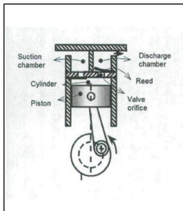
**Figure 2:** Shows the schematic and working of Reed valve in a reciprocating compressor. Adapted from “Influence of piston on effective areas of reed-type valves of small reciprocating compressors”, by E.L.Pereira, 2011, *HVAC&R Research*, 17(2): p.218-230, Copyright (2011) American Society of Heating, Refrigerating and Air-conditioning Engineers, Inc.
