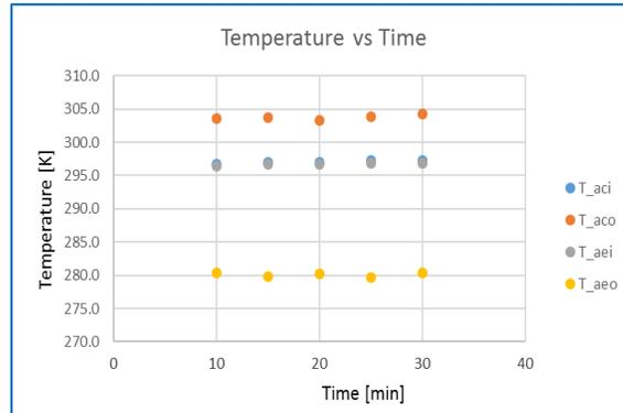
**Figure 5:** Shows the variation of temperature readings in steady state. The sensors have an accuracy of +/- 1°C. T\_aci is the temperature of the air at the condenser inlet, T\_aco is the temperature of air at the condenser outlet, T\_aei is the temperature of air at the evaporator inlet and T\_aeo is the temperature of air at the evaporator outlet.
