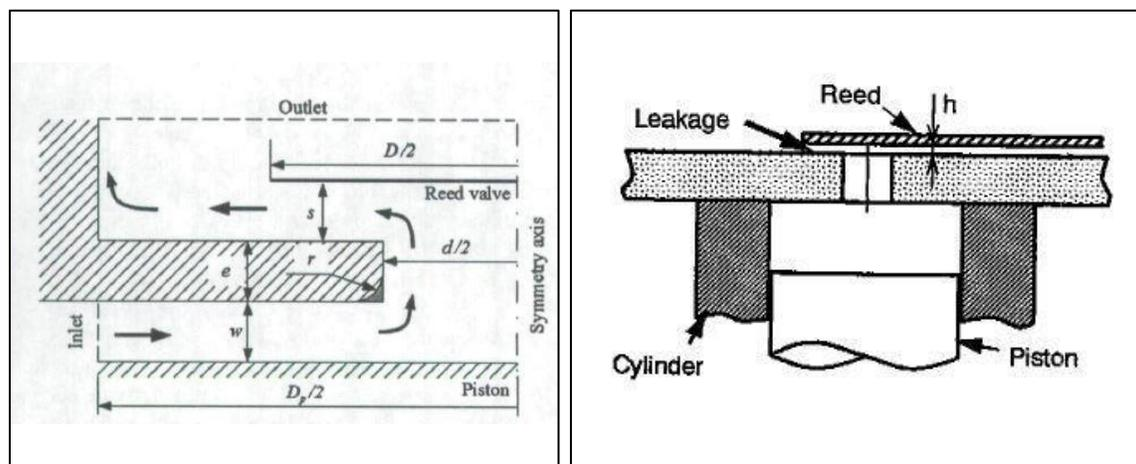
**Figure 3:** Schematic of Reed valve showing the geometry and primary design variables critical to the efficiency of compressors. Adapted from “Influence of piston on effective areas of reed-type valves of small reciprocating compressors”, by E.L.Pereira, 2011, *HVAC&R Research*, 17(2): p.218-230, Copyright (2011) American Society of Heating, Refrigerating and Air-conditioning Engineers, Inc.
