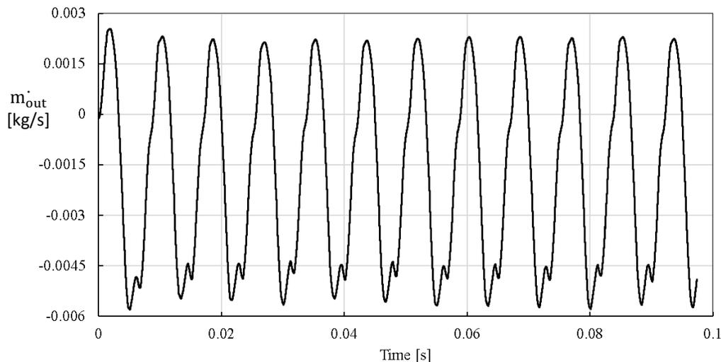
**Figure 2** Mass flow rate measured at the outlet
