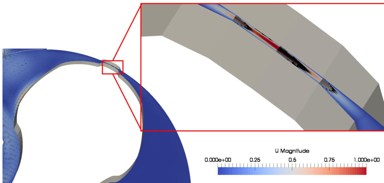
**Figure 7** Rotor-Casing gap: flow field and velocity pattern
