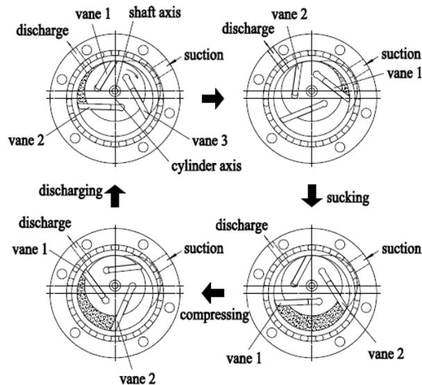
Figure 4: Compression process of HEVC
