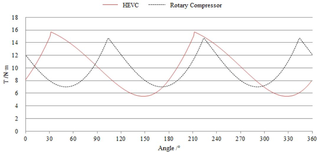
**Figure 9:** Torque comparison of two compressors
