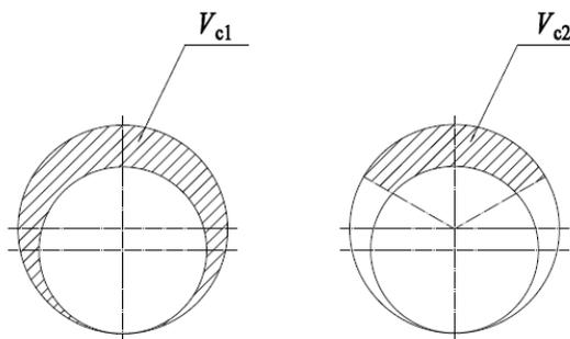
Figure 8: Volume comparison of two compressors (horizontal cross-sectional view)
