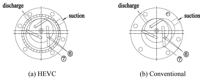
**Figure 6:** Friction locations of vane and van tip
