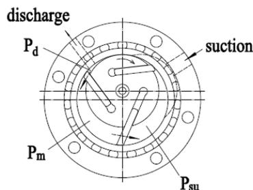
Figure 7: The model of leakage to suction
