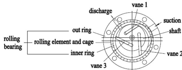
Figure 2: Basic structure of compression mechanism
