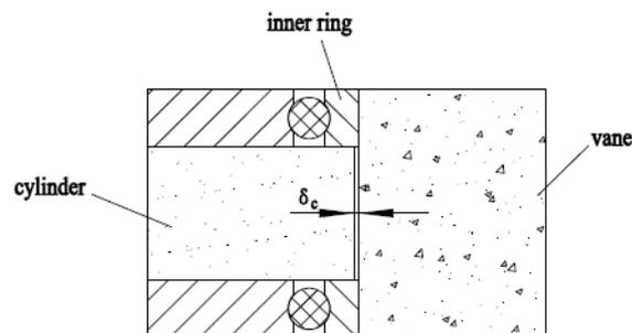
Figure 3: Assembly of the vane tip with cylinder and rolling bearing
