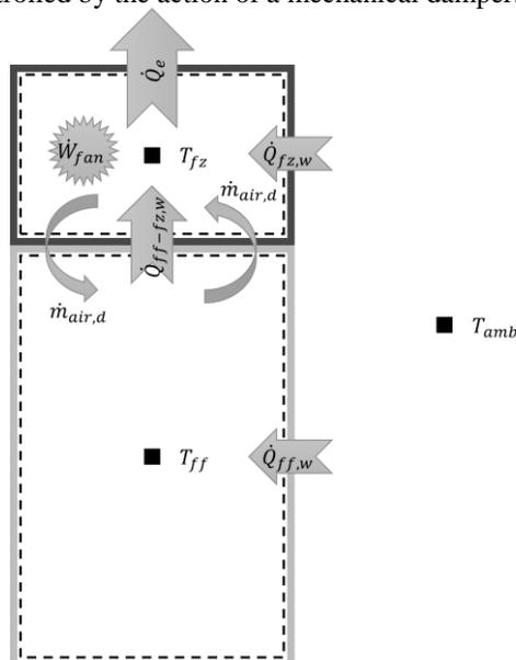
**Figure 3:** Thermal interaction of the refrigerated compartments model.
