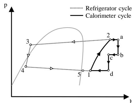
Figure 2: p-h diagram of calorimeter and refrigerator cycle.
