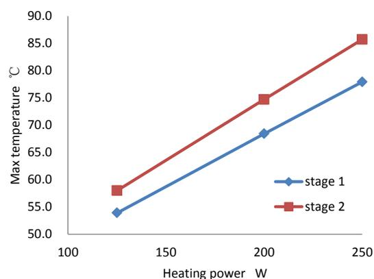
**Figure 8:** Cylinder liner wall temperature vs heating power (air temperature 30°C, air flow 60l/min)
