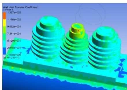
**Figure 11: convective heat transfer coefficient**
