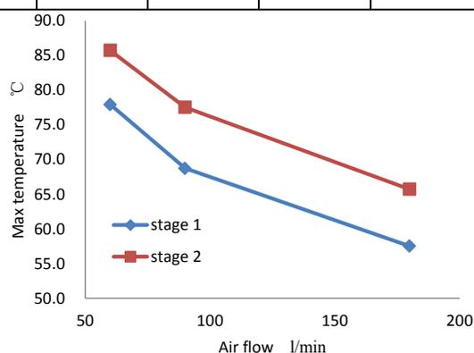
**Figure 7:** Cylinder liner wall temperature vs air flow (air temperature 30°C, heating power 250W)
