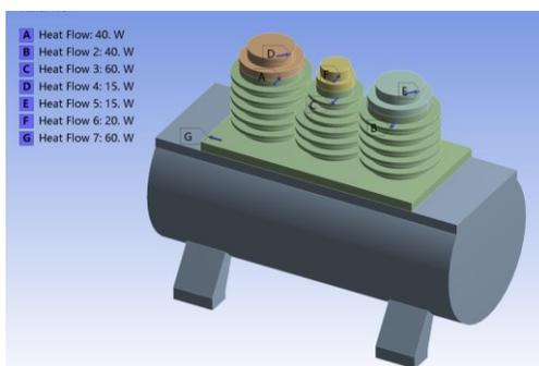
Figure 6: Heat flow boundary (250W)
