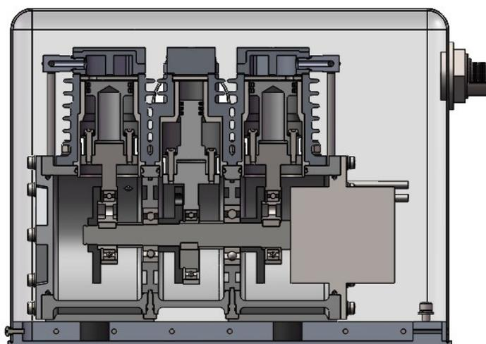
**Figure 1:** cross-section of a reciprocating compressor
