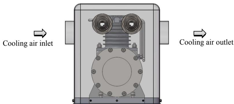
**Figure 2:** Schematic diagram of cooling air flow
