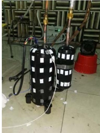
**Figure 11:** Compressor vibration test fixture
