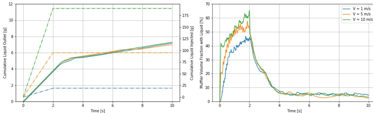
Figure 9: Liquid slugging results for muffler Design 4.
