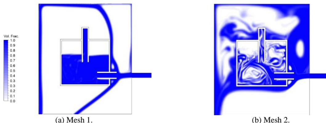
**Figure 5:** Visualization comparison of liquid fraction contours results at end of injection process, Design 1.
