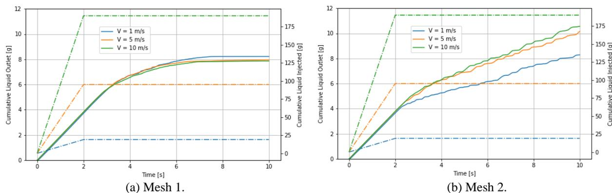
**Figure 4:** Cumulative outlet liquid mesh refinement results comparison, for Design 1.
