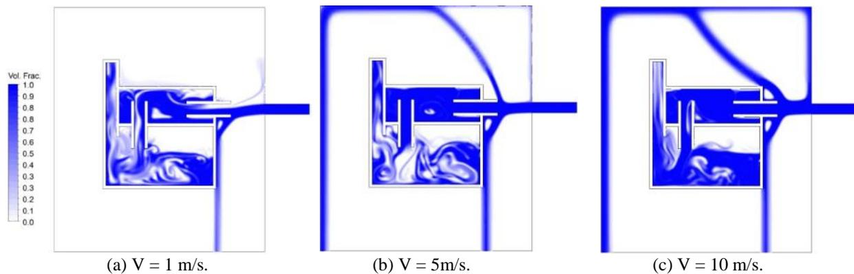
**Figure 16:** Liquid volume fraction visualization for Design 4, time 2 s.
