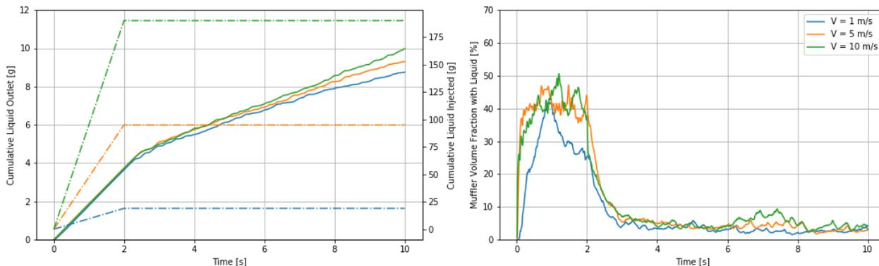
Figure 7: Liquid slugging results for muffler Design 2.
