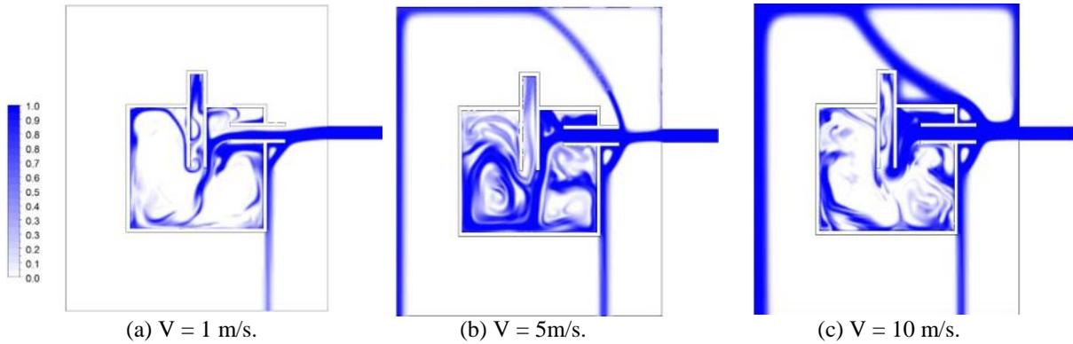
**Figure 12:** Liquid volume fraction visualization for Design 2, time 2 s.
