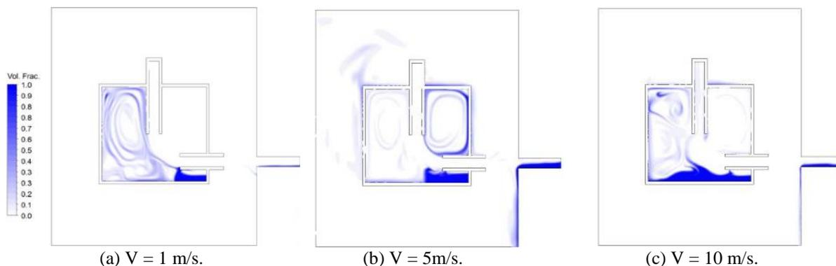
**Figure 11:** Liquid volume fraction visualization for Design 1, time 3 s.
