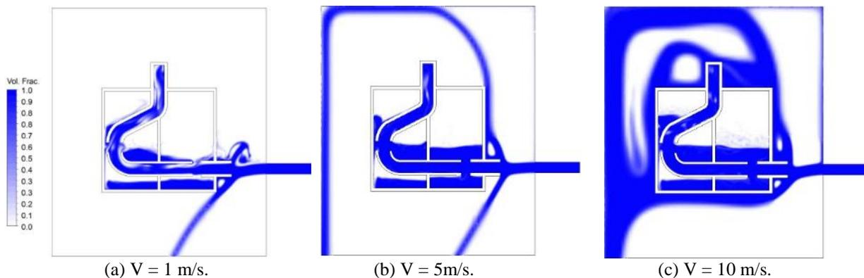
**Figure 14:** Liquid volume fraction visualization for Design 3, time 2 s.
