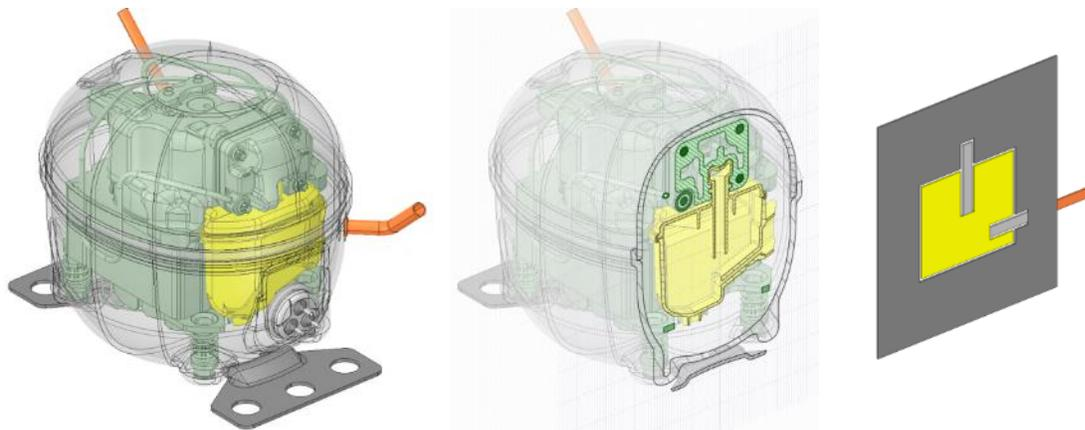
**Figure 1:** Simplification procedure, from three to two-dimensional domain.
