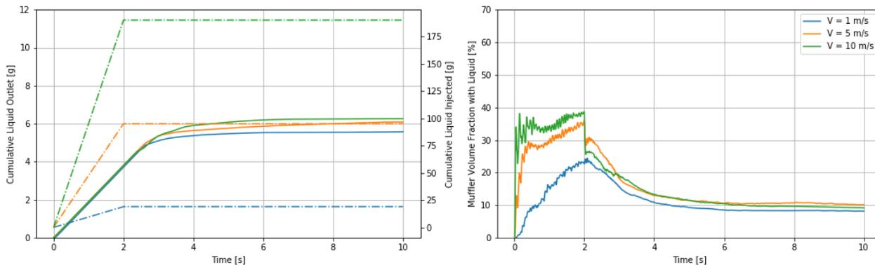
Figure 8: Liquid slugging results for muffler Design 3.
