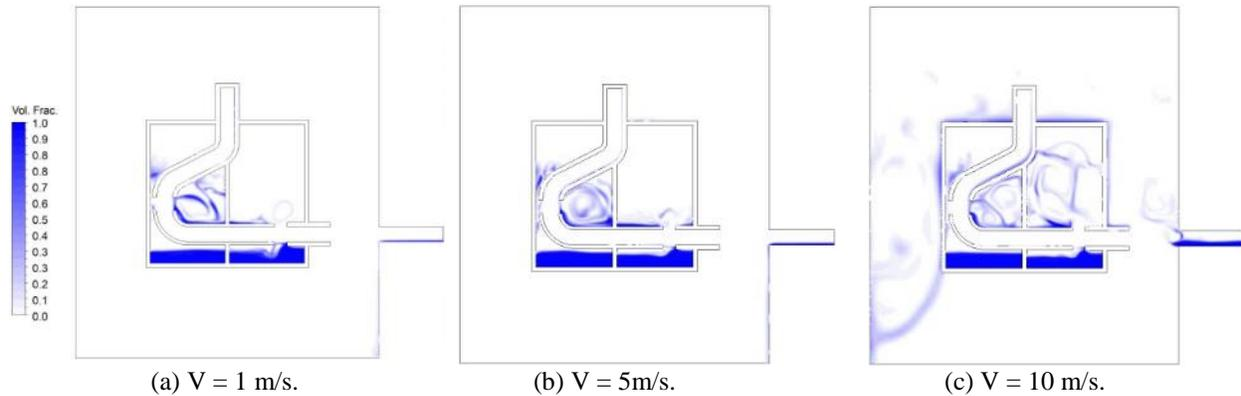
**Figure 15:** Liquid volume fraction visualization for Design 3, time 3 s.
