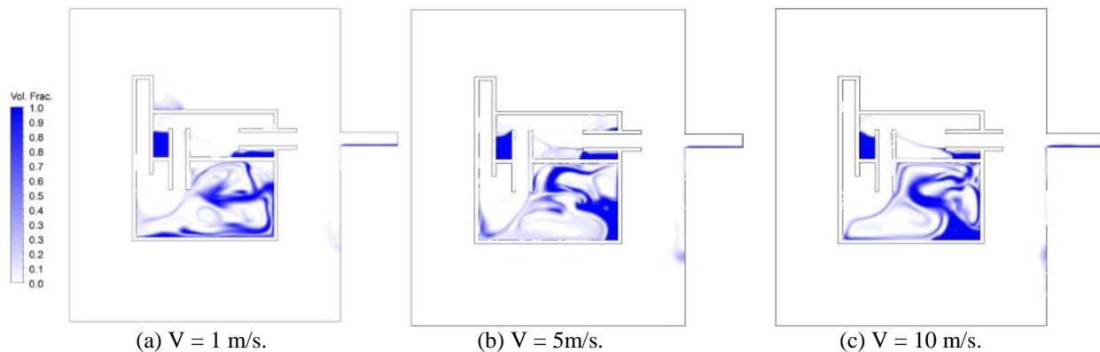
**Figure 17:** Liquid volume fraction visualization for Design 4, time 3 s.
