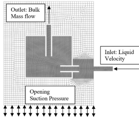
**Figure 2:** Mesh and boundary conditions used for simulations.
