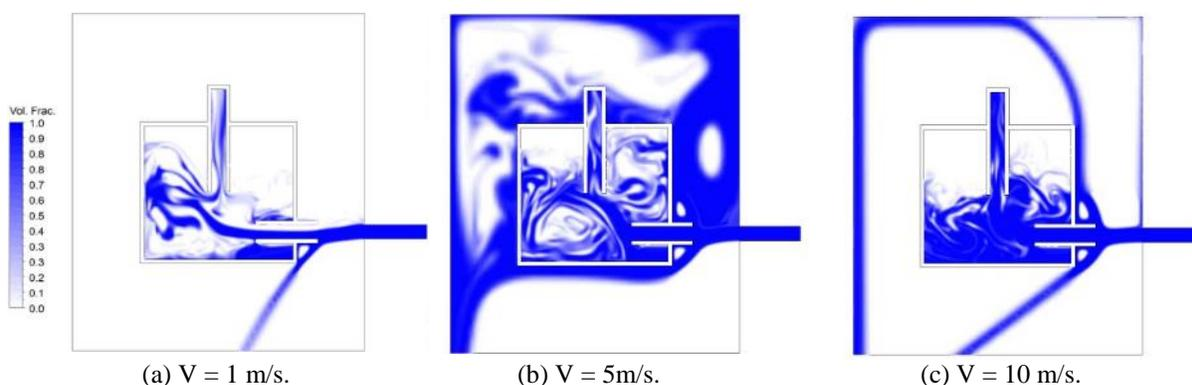
**Figure 10:** Liquid volume fraction visualization for Design 1, time 2 s.
