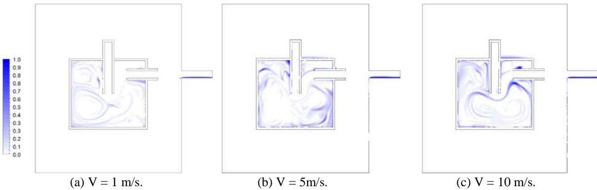
**Figure 13:** Liquid volume fraction visualization for Design 2, time 3 s.
