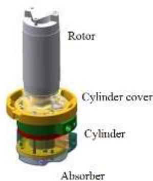
Figure 1: Schematic of shafting
