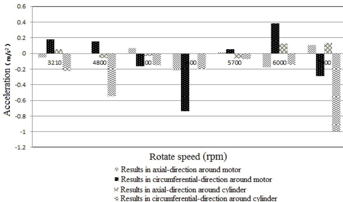
Figure 9: Normalized vibration difference between Sample 2 and Sample 3
