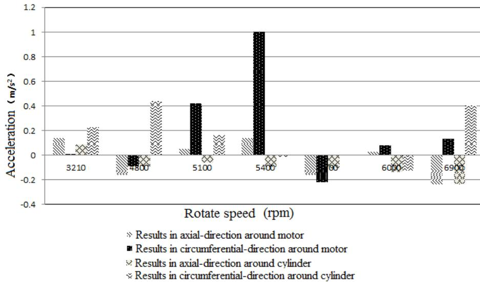
Figure 7: Normalized vibration difference between Sample 1 and Sample 2
