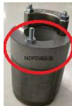
Figure 2: Photo of NOPD shock absorber sample attached on rotor
