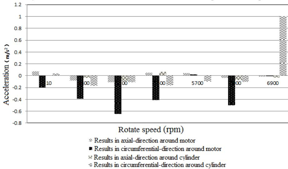
Figure 8: Normalized vibration difference between Sample 3 and Sample 4
