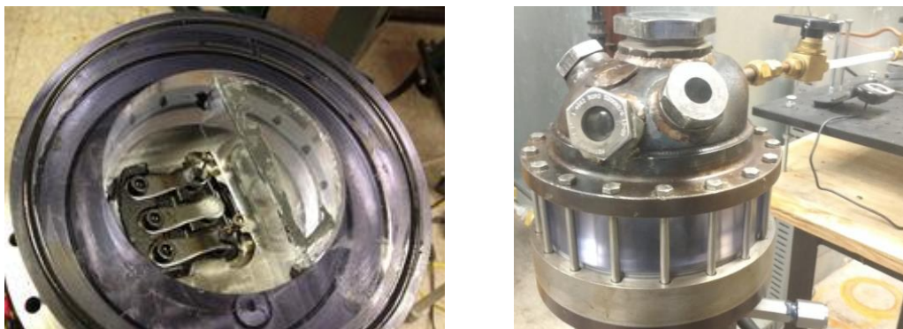
Figure 1: Modification of a scroll compressor plenum for visualization
