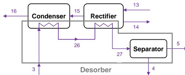
**Figure 2:** Schematic of an integrated condenser-desorber-rectifier unit of the proposed ammonia/water DL-CRHP.
