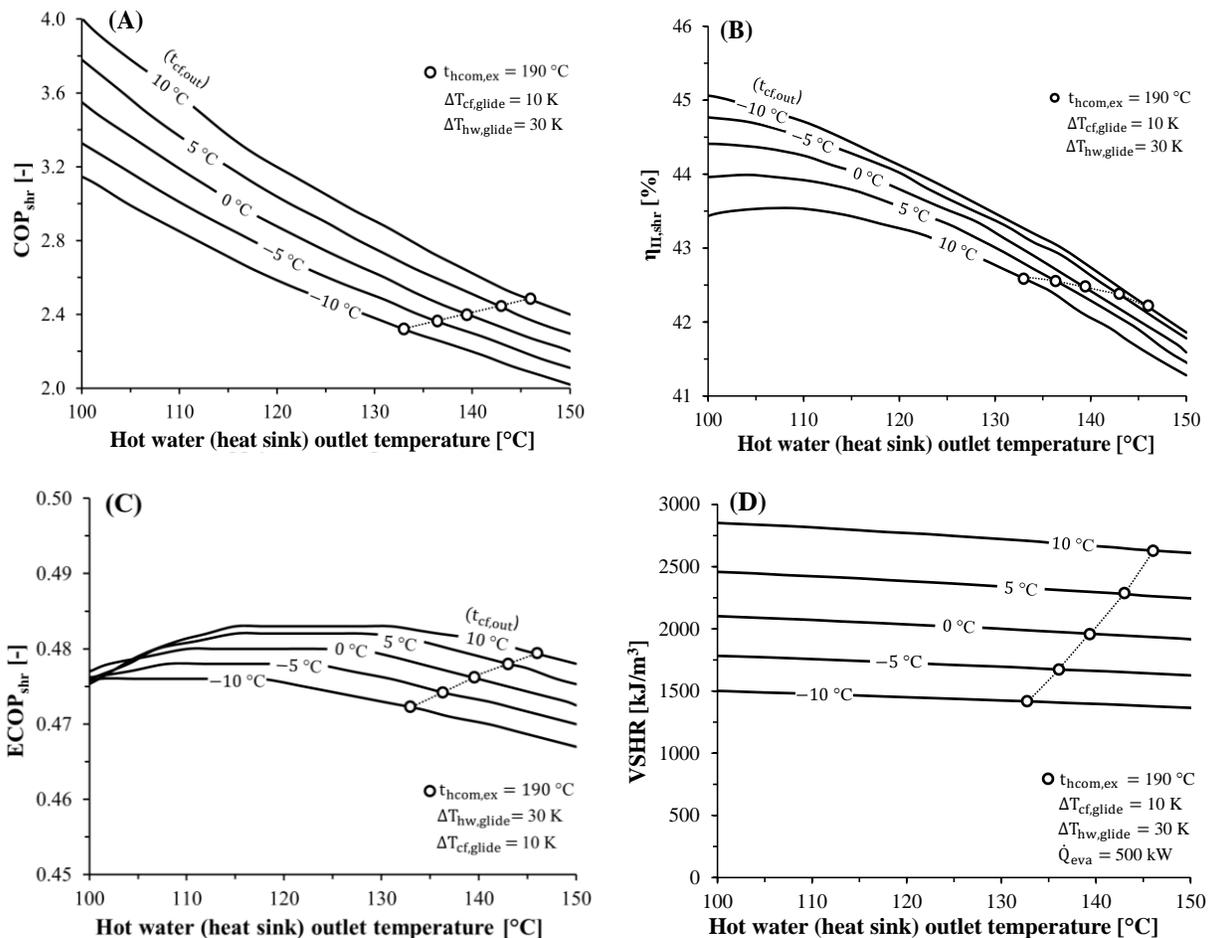
**Figure 4:** Effect of hot water (heat sink) outlet temperature on the performance of the proposed DL-CRHP. (A) combined COP ( $COP_{shr}$ ), (B) second-law efficiency ( $\eta_{II,shr}$ ), (C) exergy efficiency ( $ECOP_{shr}$ ), and (D)  $VSHR$ .
