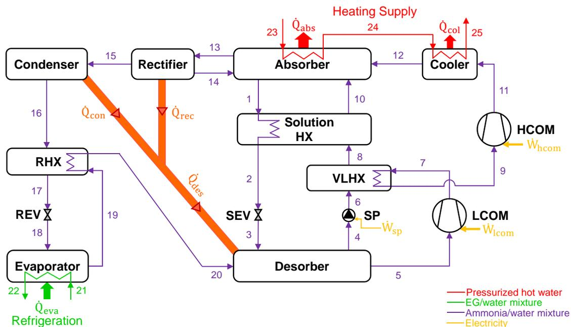
**Figure 1:** Schematic of the double-lift two-stage ammonia/water compression-resorption heat pump (DL-CRHP) cycle for simultaneous industrial process heating and refrigeration applications
