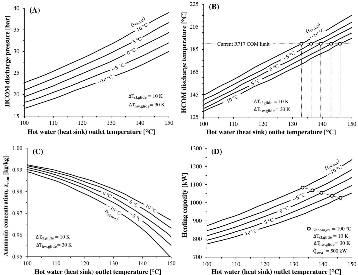
**Figure 3:** Effect of hot water (heat sink) outlet temperature on (A) high-stage compressor (HCOM) discharge pressure, (B) high-stage compressor (HCOM) discharge temperature, (C) compressed vapor ammonia concentration, and (D) heating capacity of the ammonia/water DL-CRHP.
