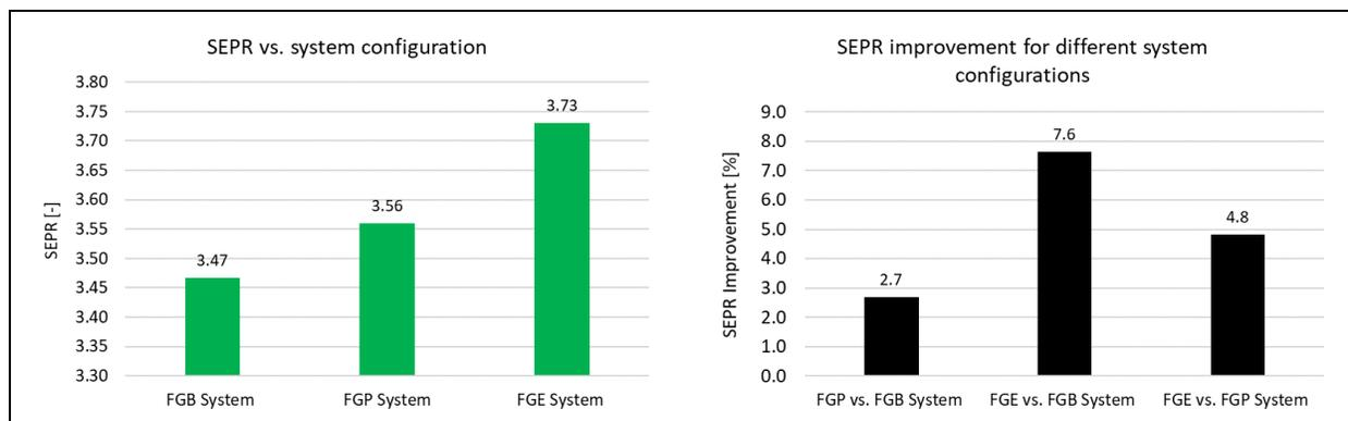
**Figure 3:** SEPR comparison for different investigated CO<sub>2</sub> Cycle Layouts
