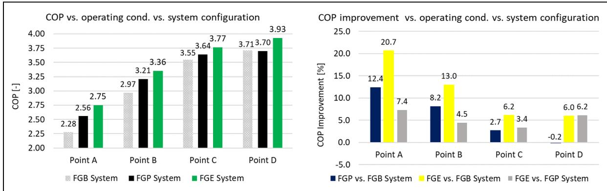
**Figure 2:** COP comparison for different investigated CO<sub>2</sub> Cycle Layouts
