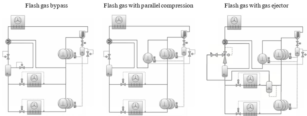
Figure 1: CO<sub>2</sub> flash gas booster systems
