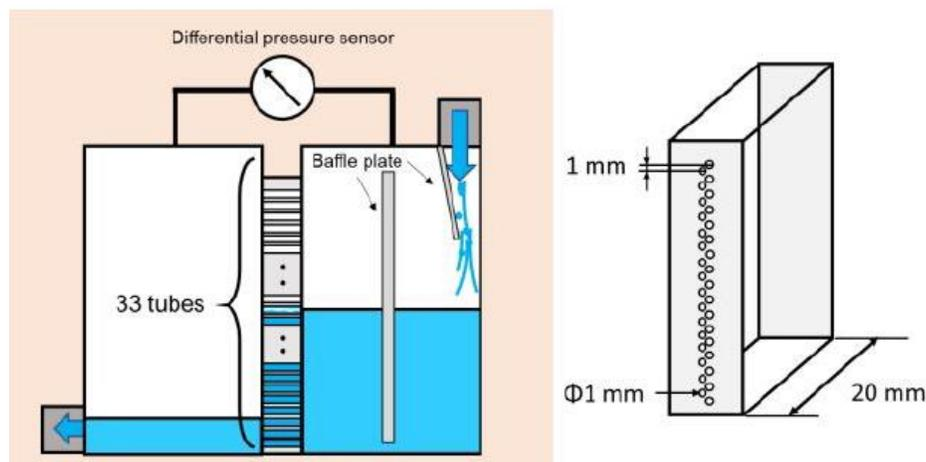
**Figure 1:** Test section with 33 passages
