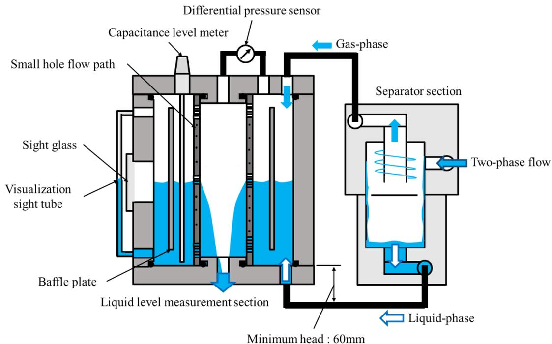
**Figure 4:** Test section
