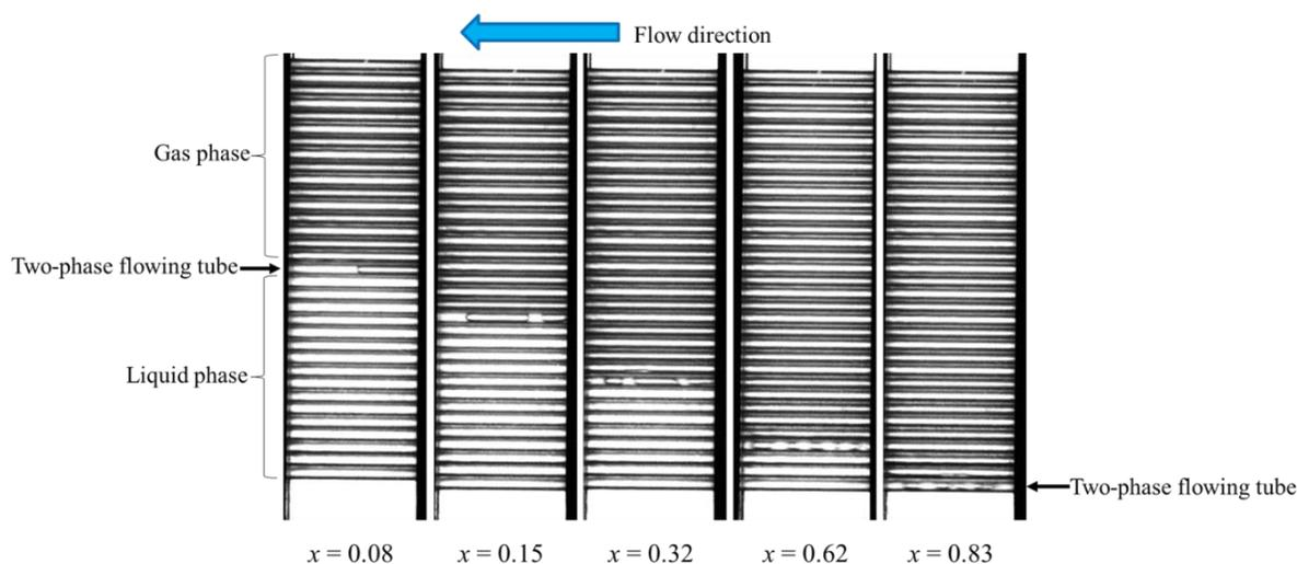
Figure 2: Flow pattern with 33 passages
