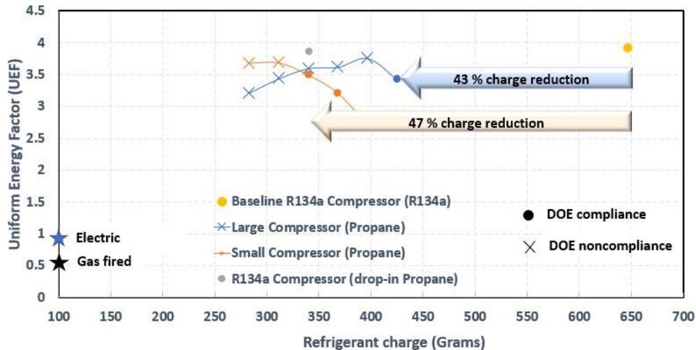
**Figure 6** UEF results for three compressors tested with propane. The baseline test with R134a is shown in yellow. The improvements of HPWH over conventional electric resistance and gas system is highlighted. The drop-in replacement of R290 with the current compressor performed the best at a much lower charge.
