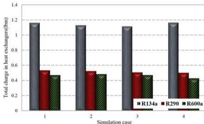
**Figure 1** Total charge in condenser and evaporator
