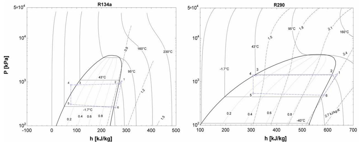
**Figure 3** Comparison of Pressure – Enthalpy diagrams for R134a (left) and R290 (right) from experimental data.
