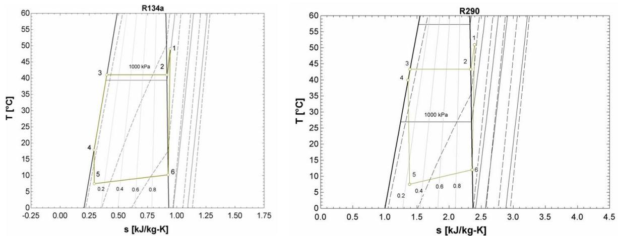
**Figure 4** Comparison of Temperature - Entropy cycle diagrams for R134a (left) and R290 (right) from experimental data.
