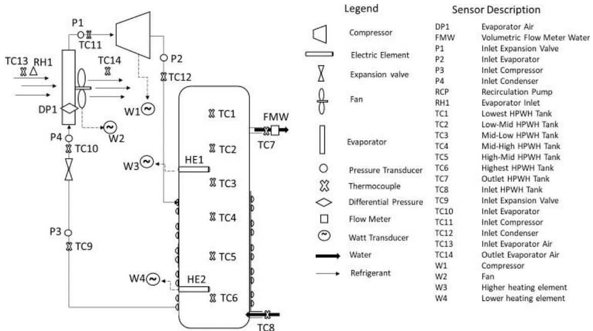
**Figure 2** Schematic of the heat pump, hot water tank, and sensor locations.
