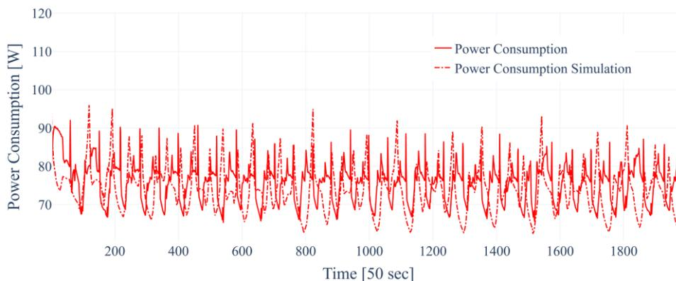
**Figure 10 Power consumption comparison between modeling and experimental results**
