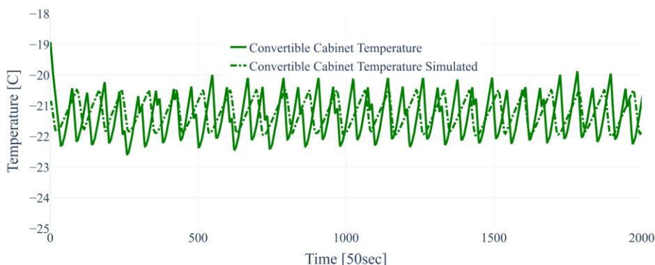
**Figure 9 Convertible cabinet temperature comparison results**
