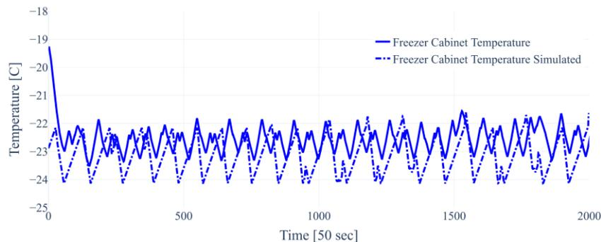
**Figure 7 Freezer cabinet temperature comparison between model and experimental results**
