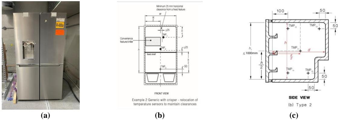
**Figure 6 Experimental set up of the experimental unit: (a) Experimental unit; (b) Refrigerator cabinet thermocouple layout; (c) Freezer/convertible cabinet thermocouple layout**
