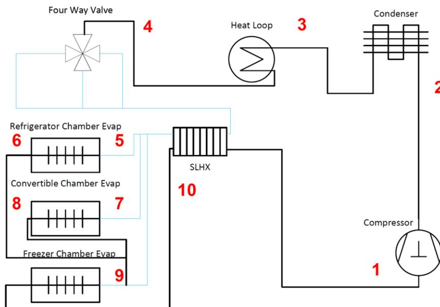
Figure 1 Schematic of the refrigerator/freezer system
