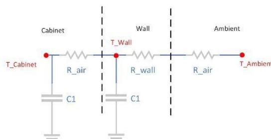
**Figure 4** Equivalent RC model of cabinet walls
