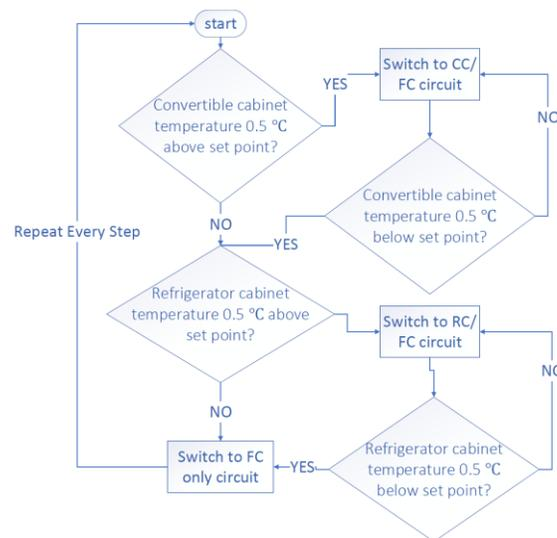
**Figure 5 Flow chart of the control logic implemented in dynamic model**
