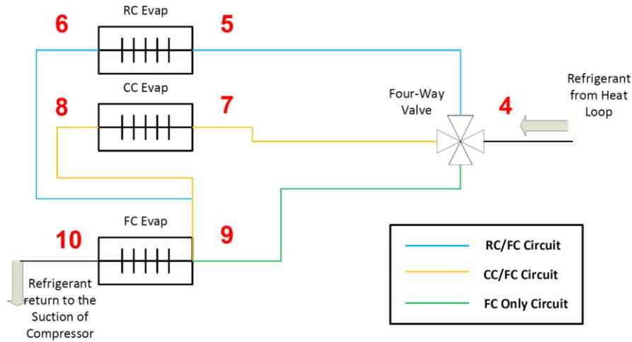
Figure 2 Illustration of the bypass circuit cycle of unit
