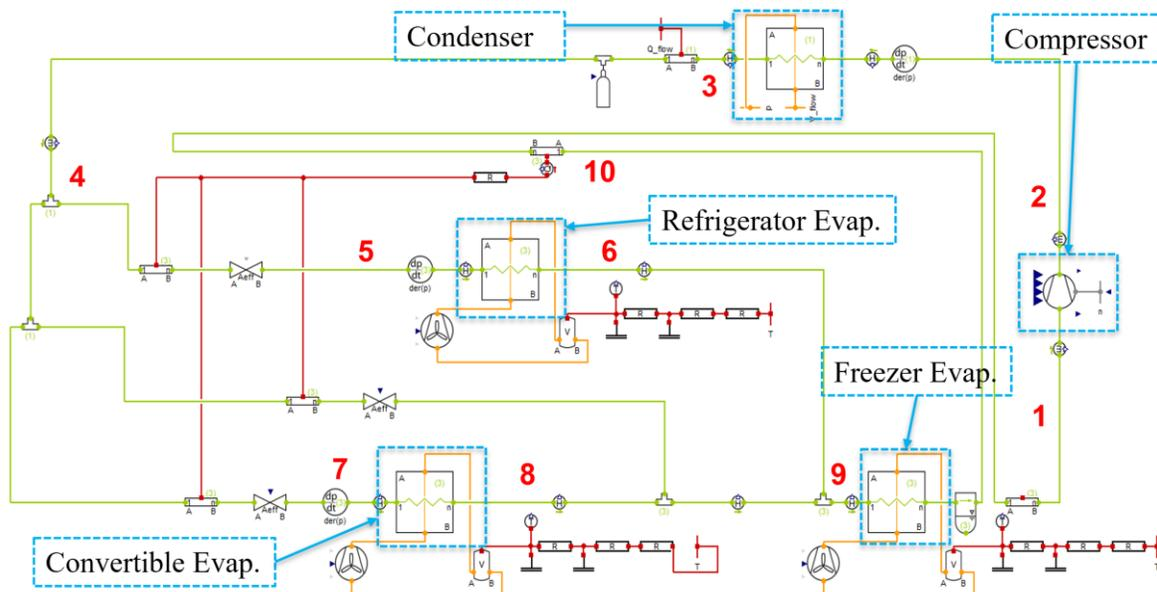
Figure 3 Triple-evaporator refrigerator/freezer system dynamic model in Dymola
