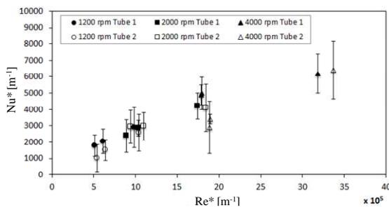
**Figure 16:** Nusselt number for tubes 1 and 2 as a function of Reynolds number.
