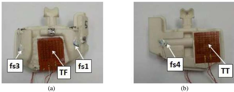
**Figure 4:** Thermocouples (fs1, fs3 and fs4) and heat flux sensors (TF and TT) on the (a) front and (b) back surfaces mufflers of group B.
