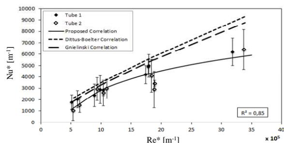
**Figure 17:** Comparison between estimates for Nusselt number given by different correlations for tubes.
