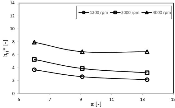
Figure 9: Heat transfer coefficients for tube 1.
