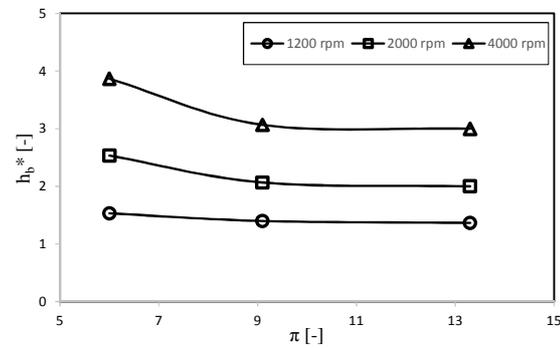
**Figure 8:** Heat transfer coefficients on the back surface of the suction muffler.
