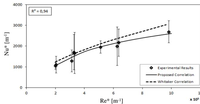
Figure 15: Comparison between correlations at the external surface.
