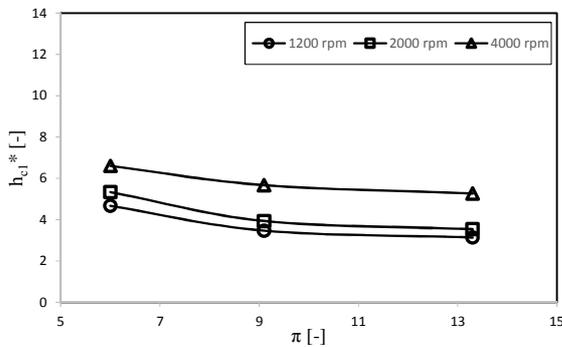
Figure 11: Heat transfer coefficients for chamber 1.
