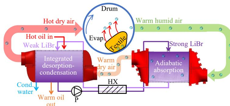
**Figure 1:** A schematic of the sorption-based dryer system.
