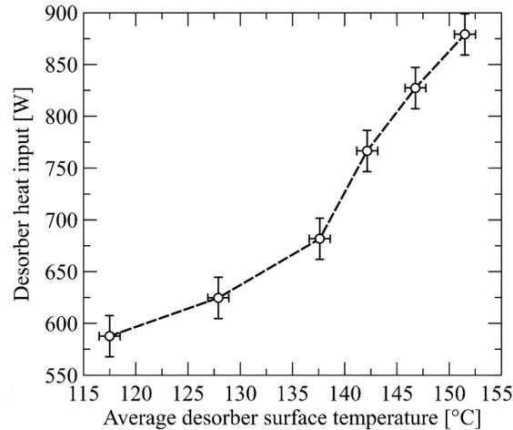
**Figure 3:** Desorber heat input versus desorber surface temperature at a constant LiBr flow rate of 4 g/s.
