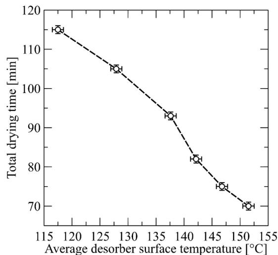
**Figure 4:** Variations of the drying time versus desorber surface temperature at a constant LiBr flow rate of 4 g/s.
