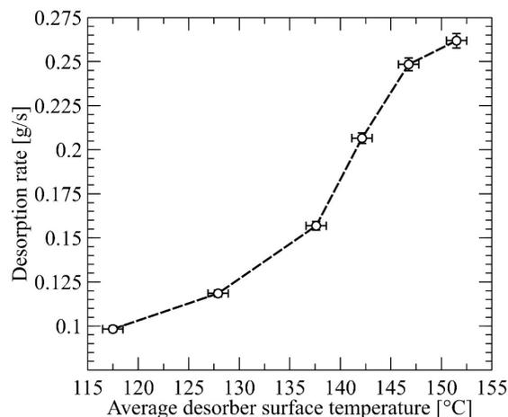
**Figure 2:** Desorption rate versus desorber surface temperature at a constant LiBr flow rate of 4 g/s.
