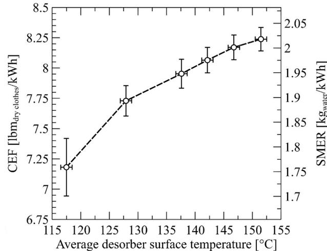
**Figure 5:** Variations of the CEF/SMER versus desorber surface temperature at a constant LiBr flow rate of 4 g/s.
