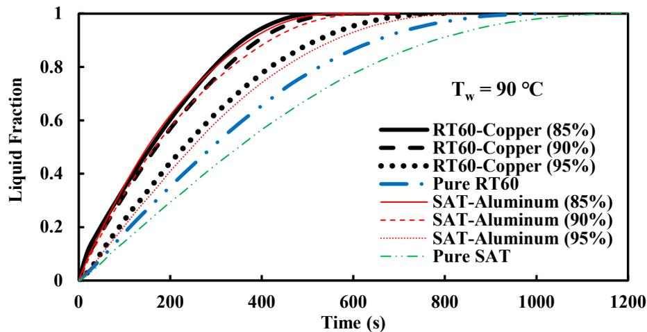
**Figure 4:** Liquid fraction variation with time at different foam porosities and different PCM-foam composites ( $T_w=90^\circ\text{C}$ )
