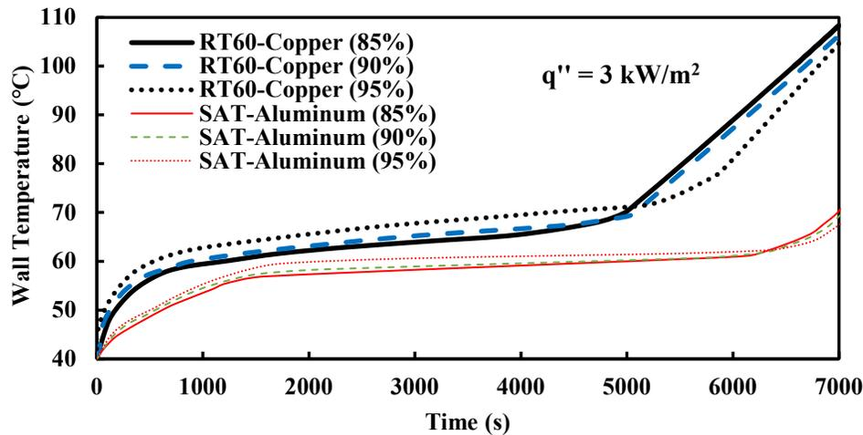
**Figure 5:** Variation of left wall temperature with time at different porosities and different PCM-foam composites ( $q'' = 3 \text{ kW/m}^2$ )
