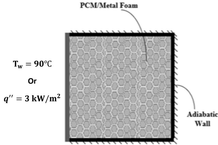
**Figure 1:** Schematic of PCM/Metal foam model
