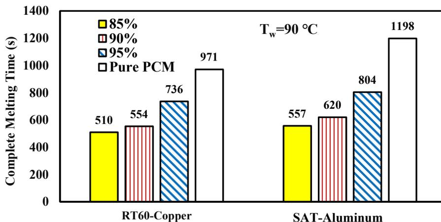
**Figure 3:** Complete melting time for different porosities and different PCM-foam composites ( $T_w=90^\circ\text{C}$ )
