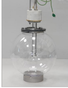
Figure 4: Polycarbonate Sphere and electrodes
