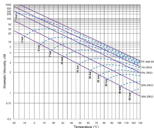
Using this data and Daniel Plot data from POE32 with R-404A a comparison was made at four different pressures and two different temperatures. The comparison data is tabulated in Table 3. Even though there could be some difference in operating conditions between the two refrigerants that might result in slight changes to the numbers, this is a good indication that when using the same POE lubricant for both R-404A and R-449A the working viscosities provided to the bearings will be similar.
