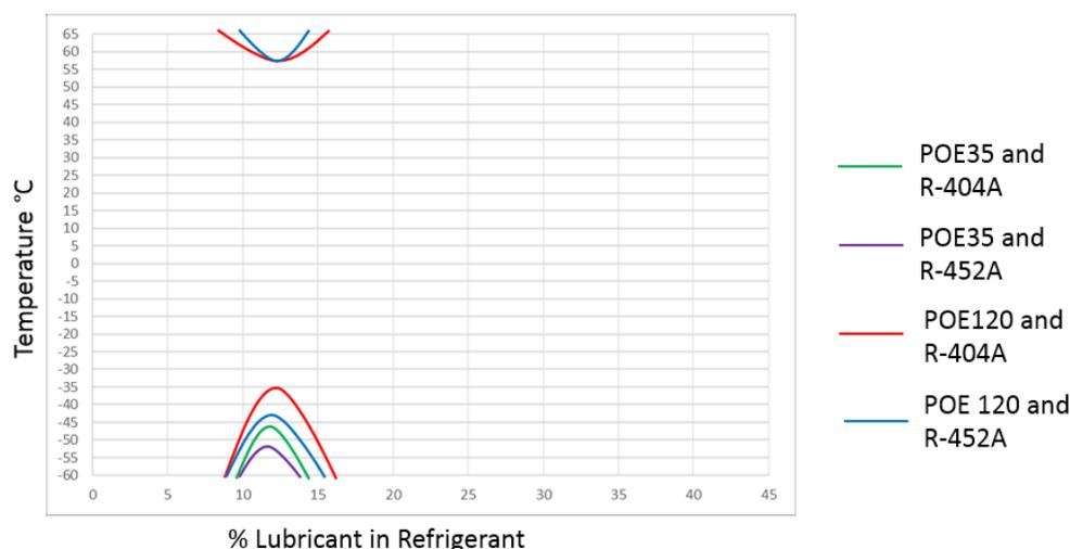
PVT data generated for the two POE lubricants listed in the miscibility tests indicated that these lubricants have similar profiles with the two refrigerants and would be considered similar enough that differences seen in compressor lubrication should also be minimal. Actually, compressor testing was done to confirm what was measured in the PVT data and no issues were reported.
