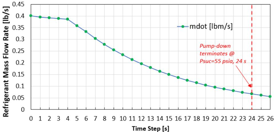
Figure 10: Transients of mass flow rate in compressor
