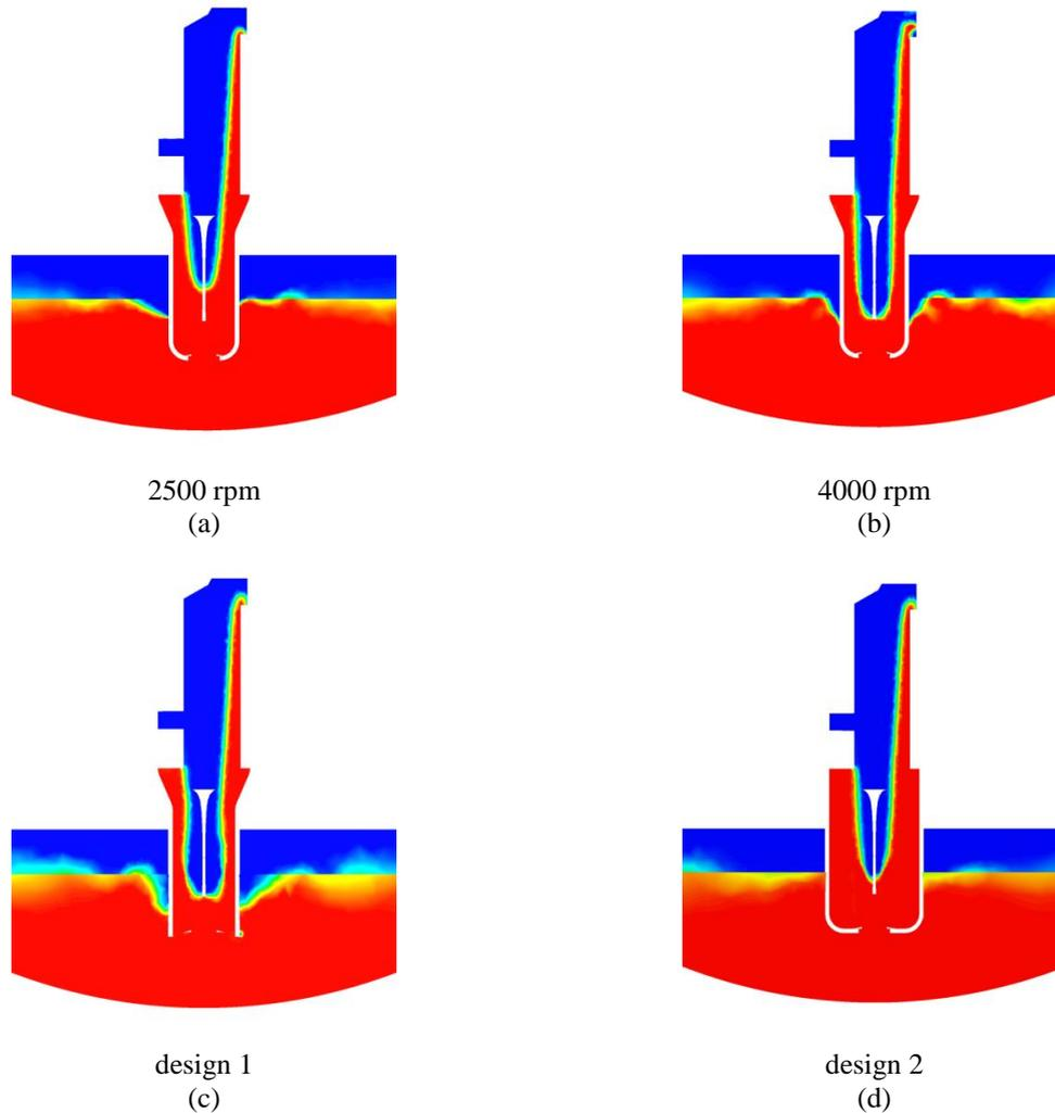
**Figure 3:** Steady-state oil volume fraction
