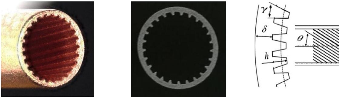
Figure 5: Photography and schematic view of the microfin tube
