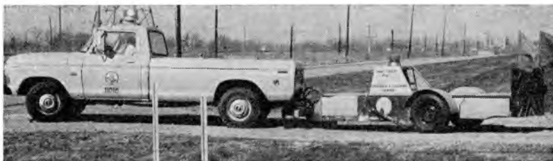
Figure 1. The Indiana State Highway Commission Skid Testing System
