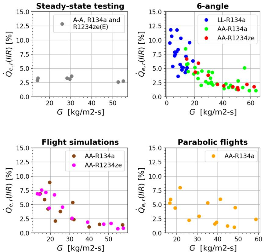
Figure 4: IIR of refrigerant side evaporator heat transfer rate for all datasets.
