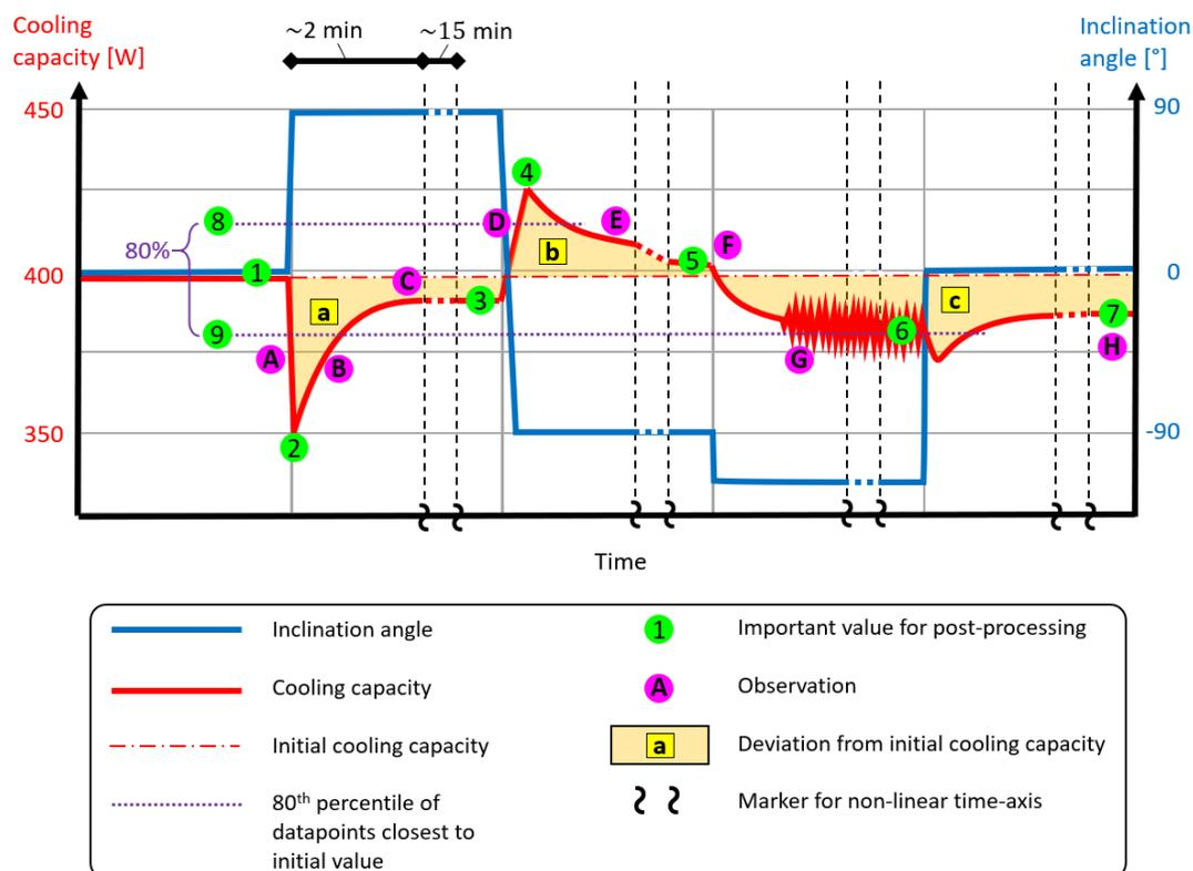
Figure 3: Example cycle responses to inclination angle changes.
