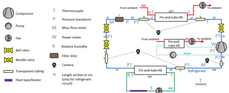
Figure 1: Schematic of refrigeration cycle test stand in air-to-air configuration.
