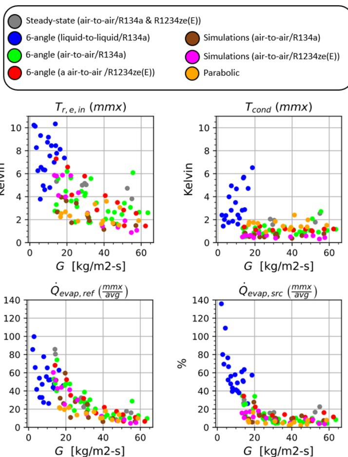
Figure 5: MMX and MMX/AVG quantifier for all testing series.
