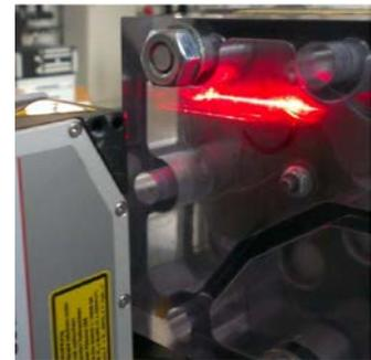
**Figure 7:** Application of a laser profile scanner for valve lift measurements
