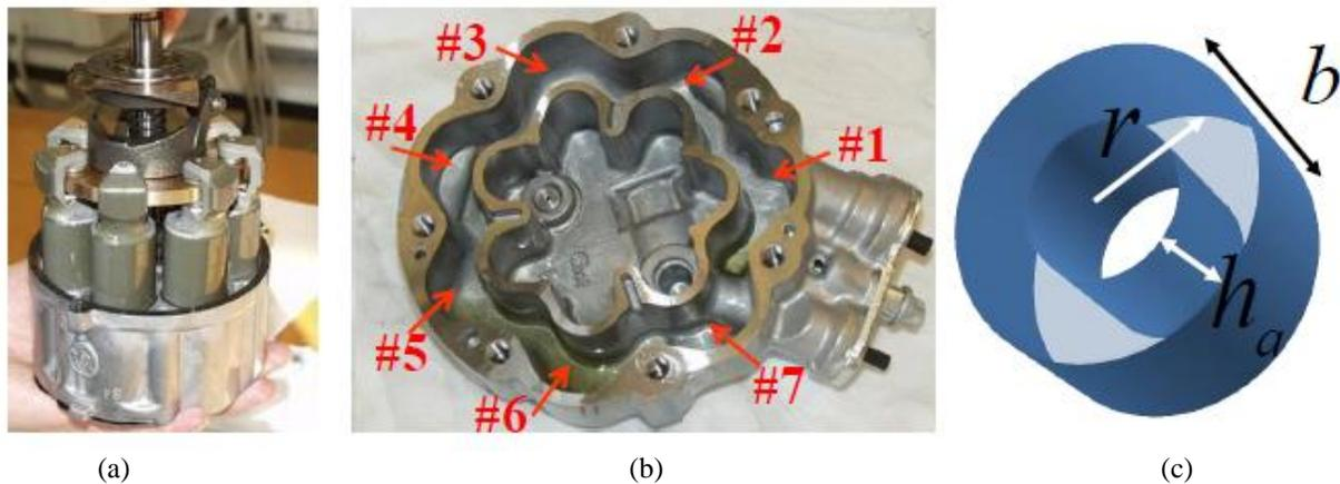
**Figure 1:** (a) A multi-cylinder reciprocating compressor and; (b) the suction manifold of the compressor with suction valves marked; (c) simplified geometric representation of the suction manifold, where  $r$ ,  $b$ , and  $h_a$  respectively represent radius, depth and width of the suction manifold.
