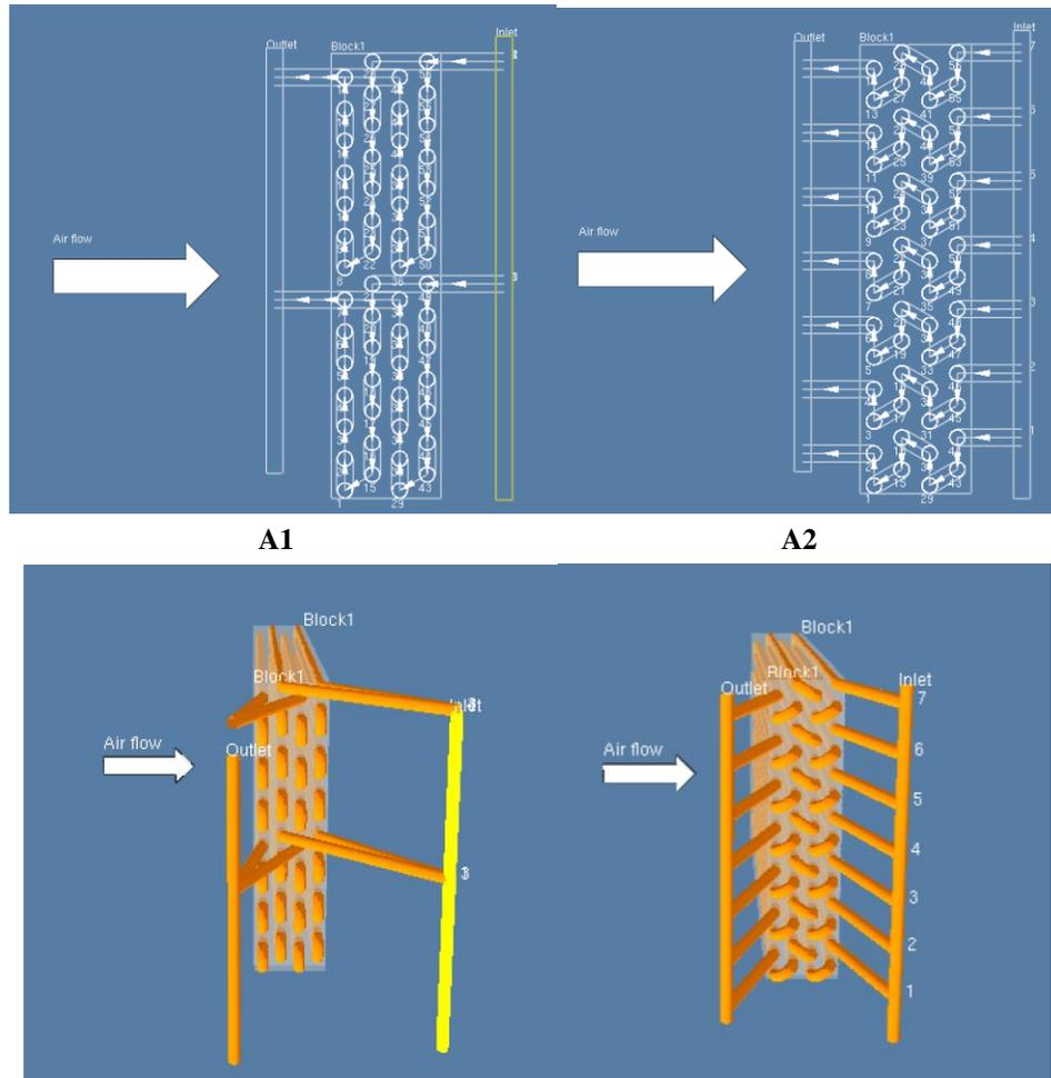
**Figure 2:** Circuit designs (top) and simulation results (bottom) of A-Series of 5 mm condenser with 52 tubes.
