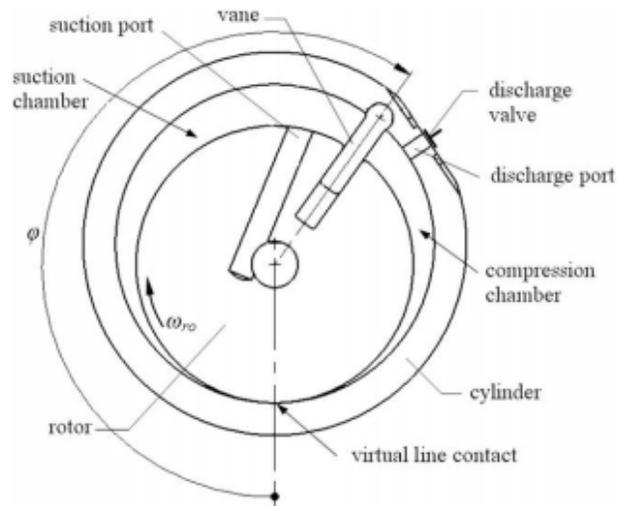
**Figure 6** Basic concept of revolving vane compressor [8]
