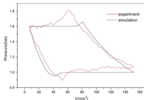
**Figure 3** Comparison of the measured and the predicted P-V histories [1]
