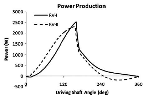
**Figure 12** Power production of a Revolving vane expander [34]
