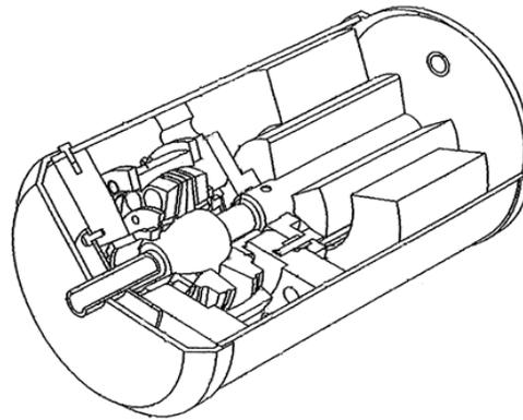
**Figure 10** Twin plate rotary compressor
