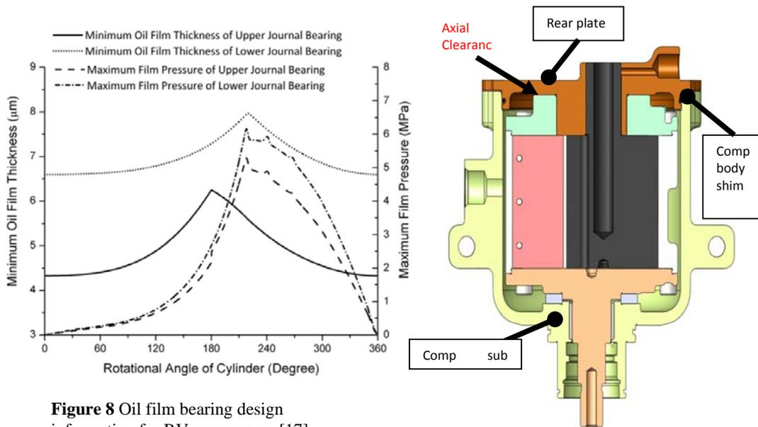
Figure 8 Oil film bearing design information for RV compressor [17]
