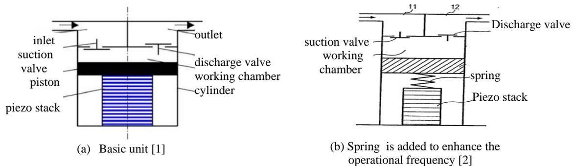
**Figure 1** Schematic of the piezo-compressor [1,2]
