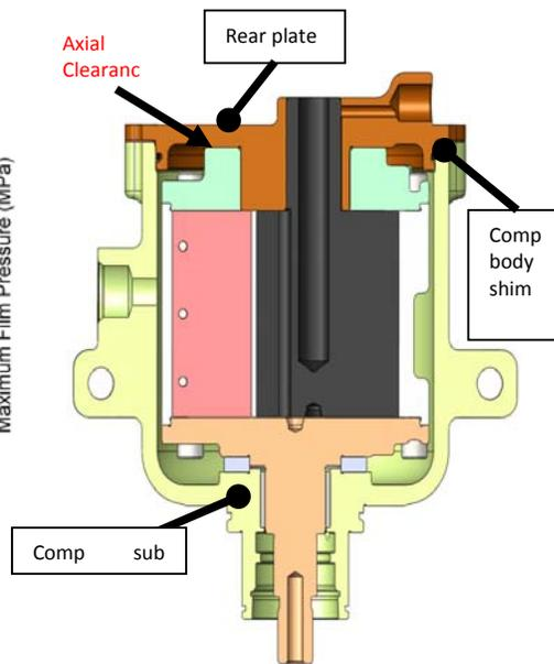
Figure 9 Revolving vane compressor for automobile applications [27]
