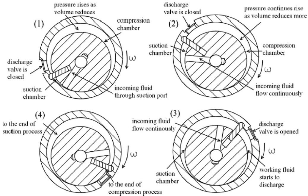
Figure 7 Snapshots of the operation of the revolving vane compressor [16]
