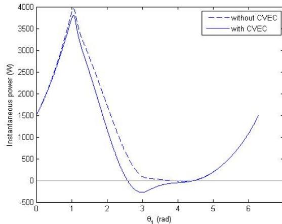
Figure 15 Variation of instantaneous power for a CVEC [43].
