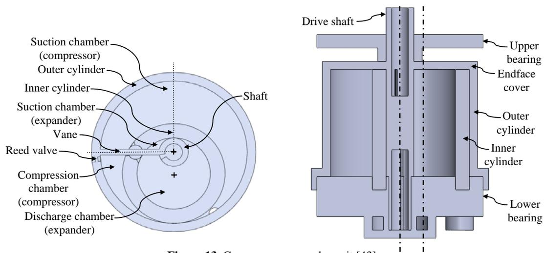
Figure 13 Compressor-expander unit [43]
