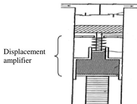
**Figure 2** A piezo compressor with a displacement amplifier [3,4]
