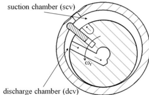
**Figure 11** Revolving vane expander [30]
