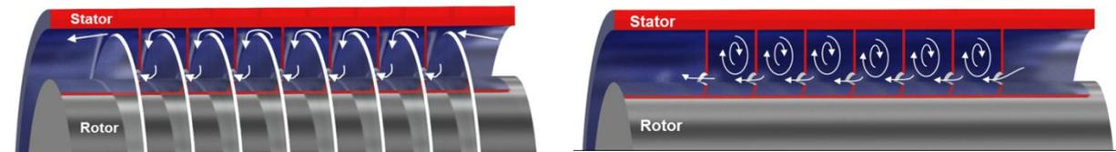
**Figure 2:** Full labyrinth (left) and transparent labyrinth (right)
