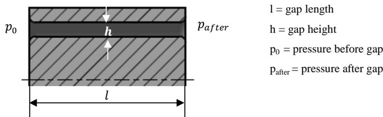
**Figure 1:** Sealing gap
