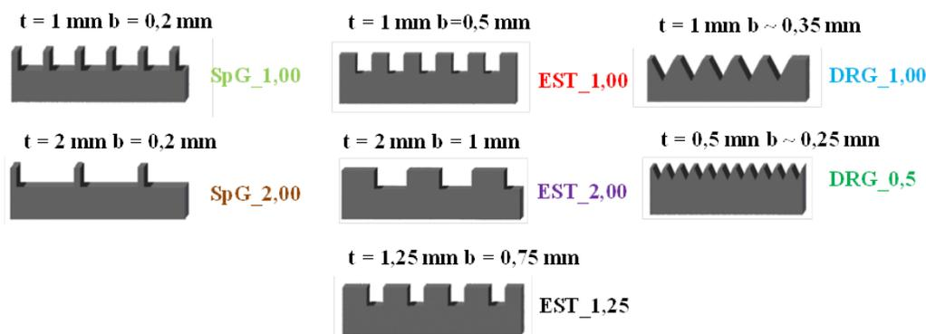
**Figure 3:** Schematic diagram of sealing variations investigated (sample)
