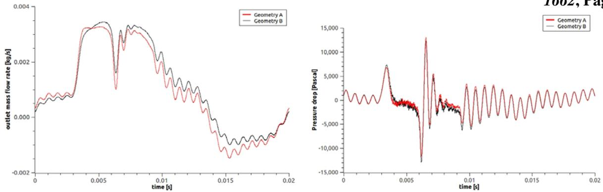
**Figure 9.** Mass flow rate at the outlet of the muffler for the two configurations (left), and instantaneous pressure drop across the muffler over one cycle (right).
