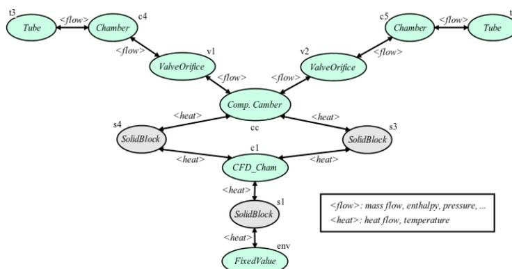
**Figure 2.** The compressor as a set of elements exchanging *flow* and/or *heat* information between each other.
