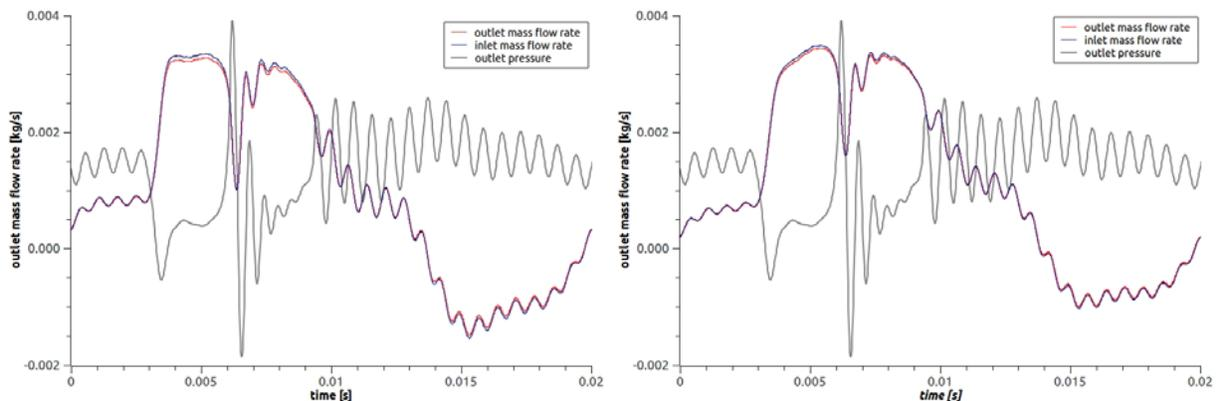
**Figure 11.** Inlet and outlet mass flow rate, superimposed on the outlet pressure for A (left) and B(right).
