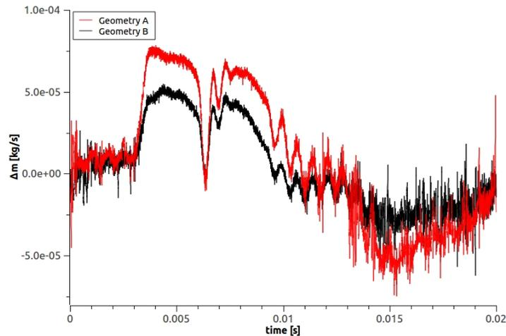
**Figure 10.** Mass accumulation inside the muffler over one cycle
