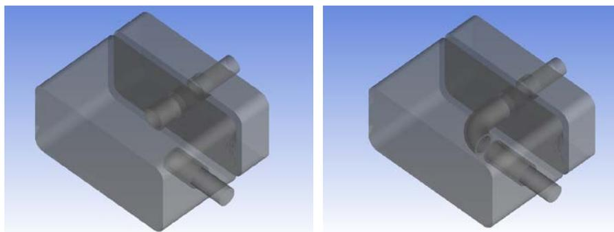
**Figure 3.** Muffler geometry (a) indirect (b) direct fluid flow from first chamber to second chamber.
