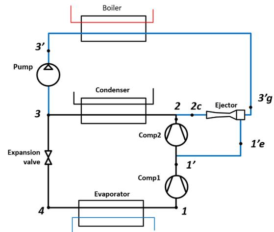
**Figure 2:** ejector booster refrigeration system
