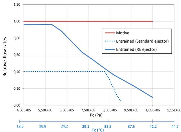
**Figure 1:** motive and entrained flow rates for standard and RE ejectors (Ortego Sampedro, 2022)
