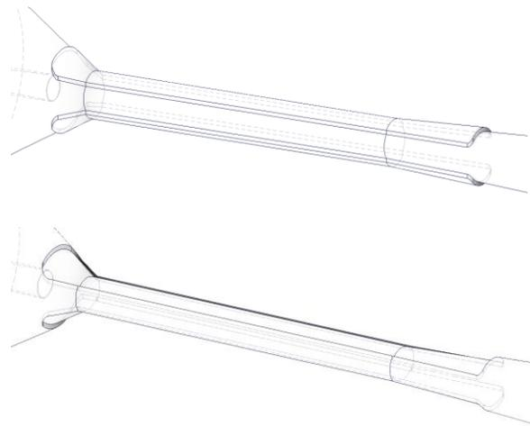
**Figure 3:** internal volume of the modified ejector: upper: 0.5mm opened extender; lower: 0.5mm closed extender
