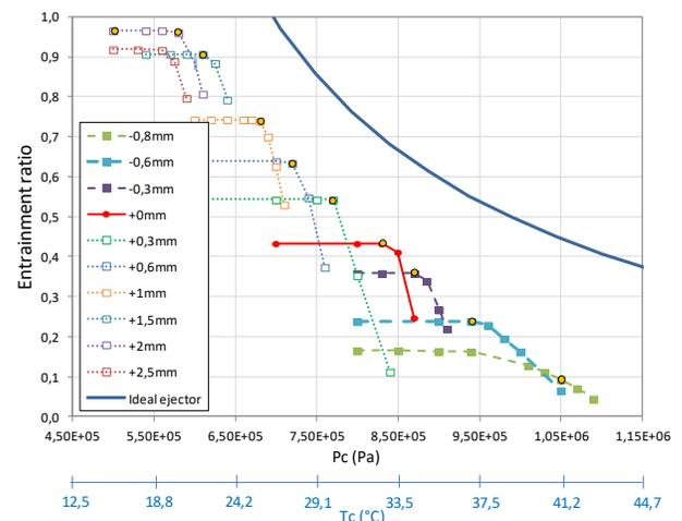
**Figure 4:** entrainment ratio function of outlet pressure the corresponding condensation temperature;  $T_{sat\ 3/g} = 84,4^{\circ}\text{C}$ ;  $T_{sat\ 1/e} = 10^{\circ}\text{C}$ ; 10 extender positions
