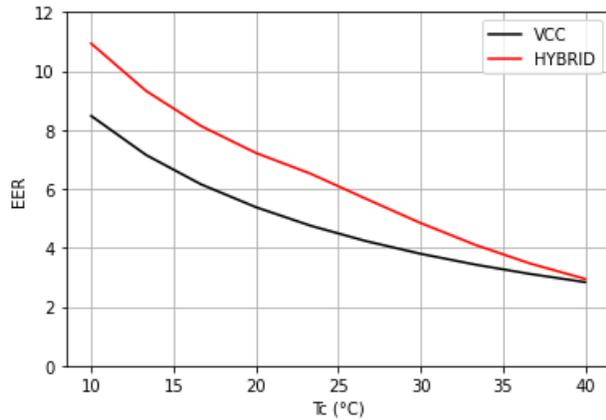
**Figure 5:** EER function of  $T_c$  at  $T_e = -10^\circ\text{C}$
