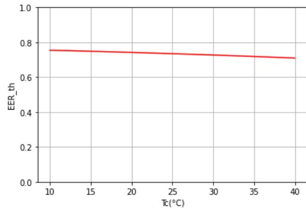
**Figure 6:** hybrid system  $EER_{th}$  function of  $T_c$  at  $T_e = -10^\circ$
