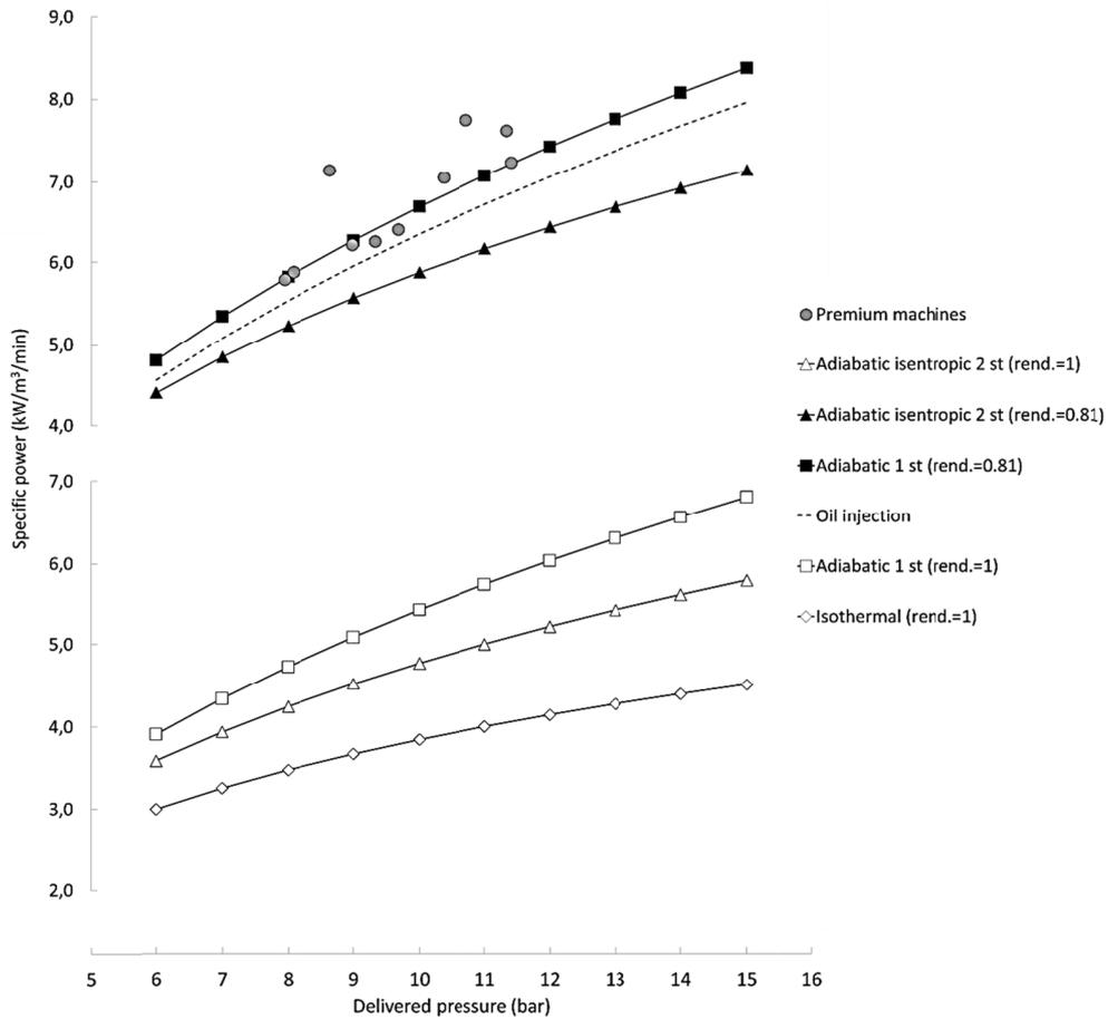
**Figure 5:** Fixed speed, Air cooled (approx. efficiency=0.81)
