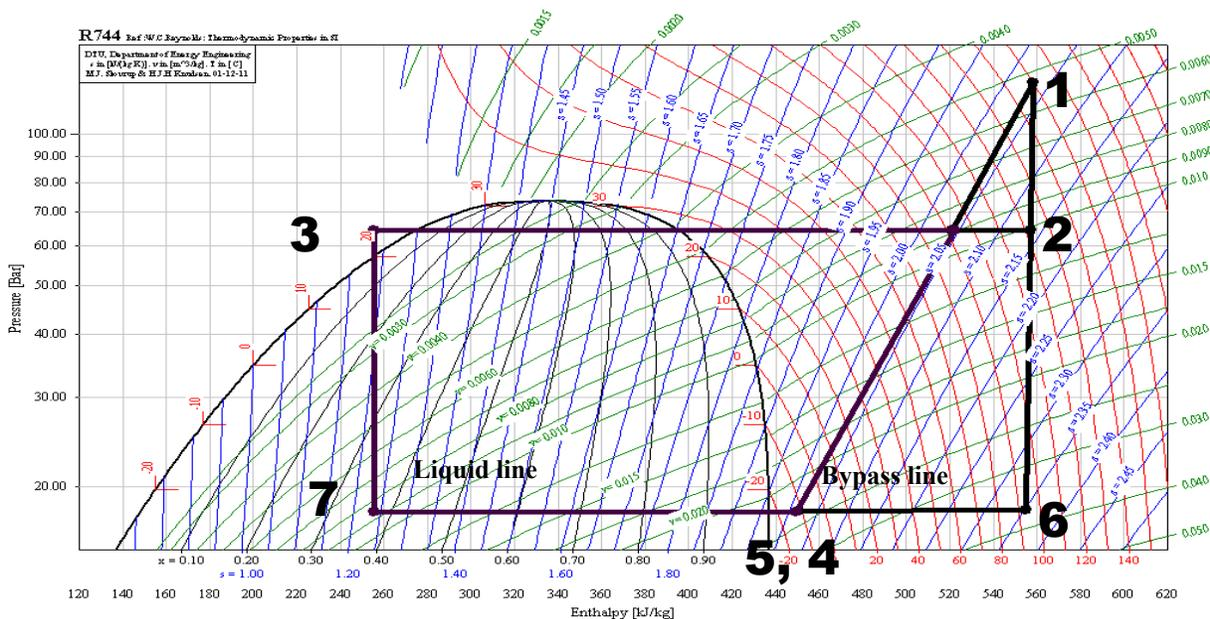
Figure 3: Load stand cycle in a P-h diagram
