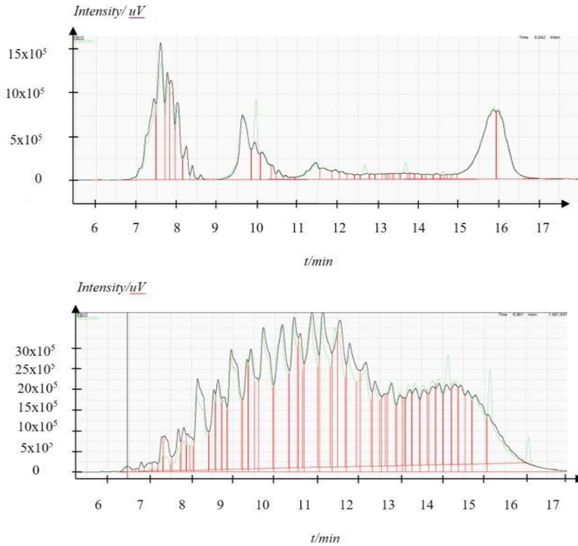
**Figure 3:** GC-SIMDIS Results for 9 cSt, 7 cSt and 5 cSt oil with their used version
