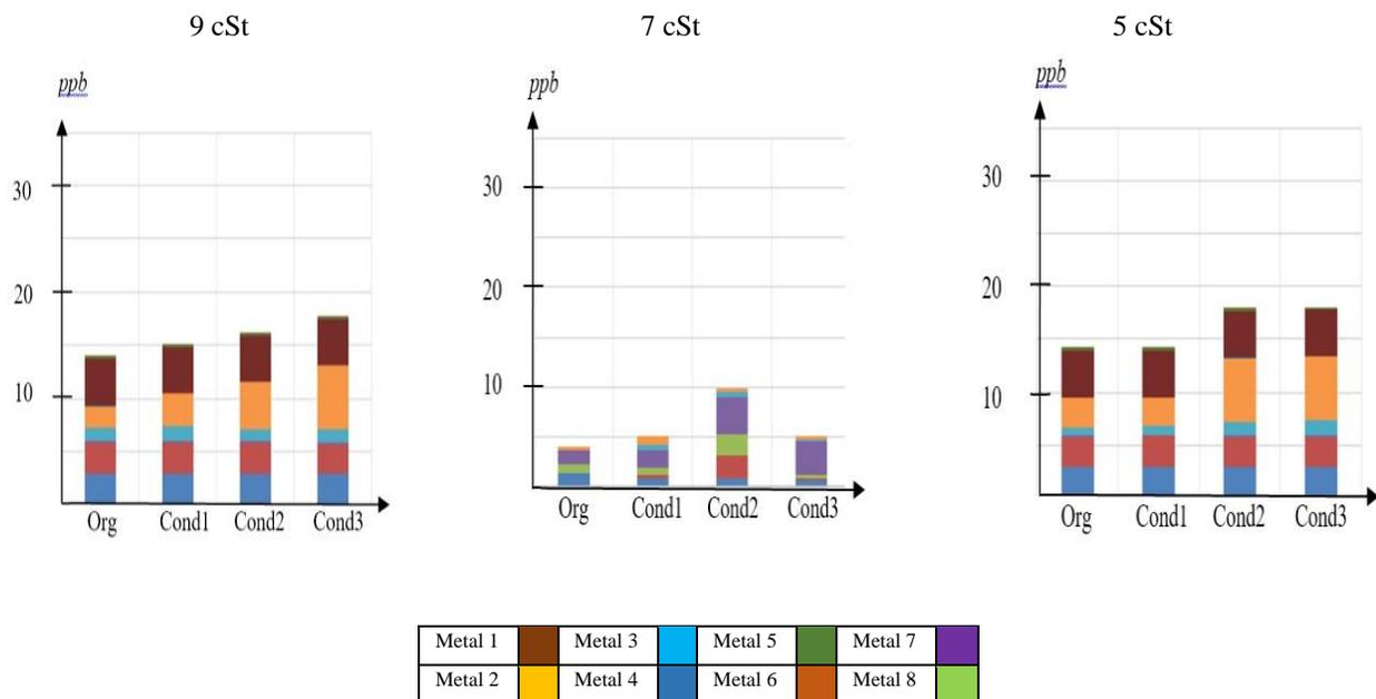
**Figure 4:** ICP-MS metallic contents results
