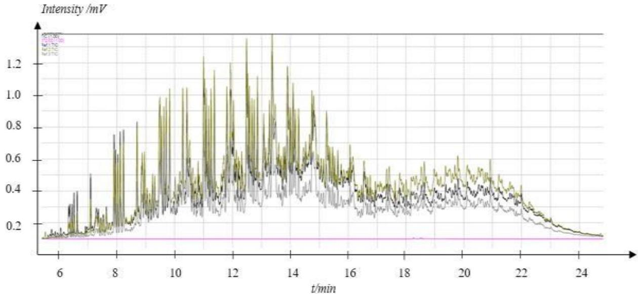
**Figure 2** : GC-MS Results for 9 cSt, 7 cSt and 5 cSt oil with their used version
