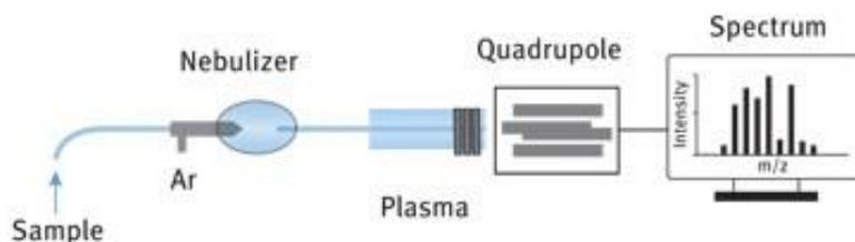
**Figure 1** : Systematic diagram for ICP by Telgmann (2016)
