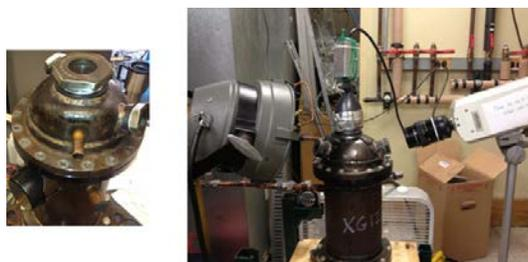
**Figure 2:** Compressor equipped with sight glasses and visualization set up
