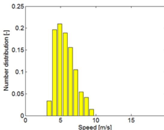
**Figure 14:** Drop speed distribution in the plenum for PVE32 oil at 50Hz.
