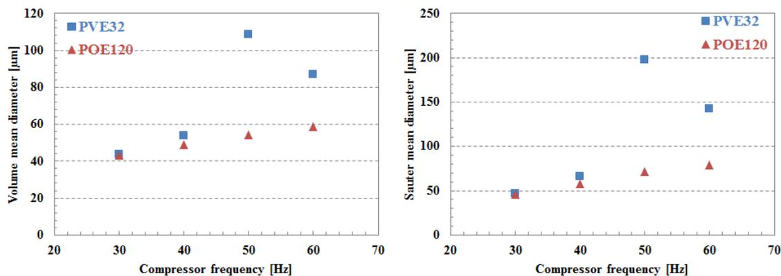
Figure 12: Volume mean diameter and Sauter mean diameter for the discharge plenum
