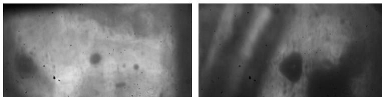
**Figure 13:** Frame from the videos for the 50Hz and 60Hz operations showing unusually large droplets most likely dripping from the top walls of the discharge cover causing the mean diameters to increase with frequency, picture dimensions are 8.63mm x 4.31mm.
