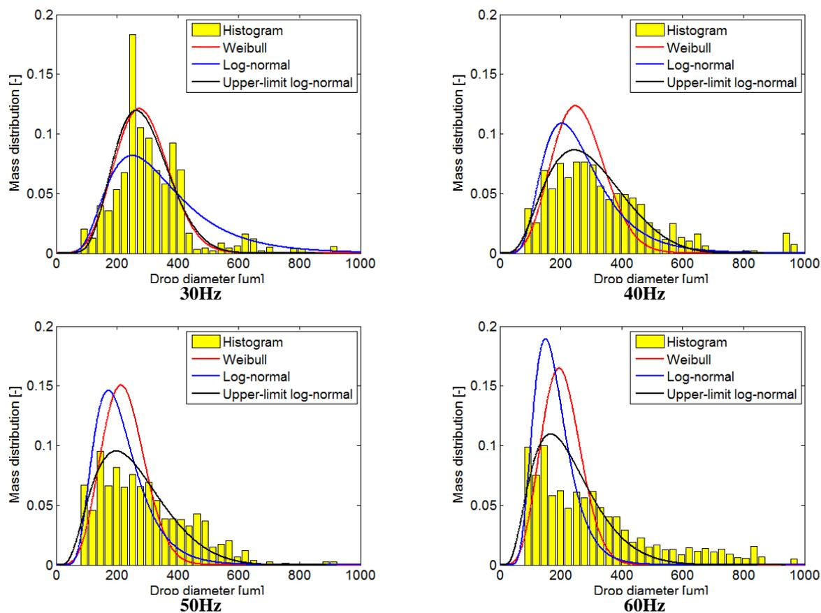
**Figure 10:** Droplet size distribution functions for POE120 oil
