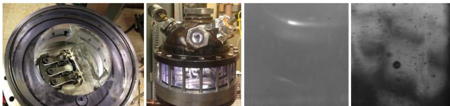
**Figure 5:** Visualization setup: transparent flange and glass barrier to enhance optical access to the valve and sample images for the valve vicinity and the discharge plenum.
