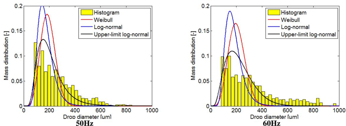
**Figure 9:** Droplet size distribution functions for PVE32 oil: smaller droplets as compressor frequency increases.
