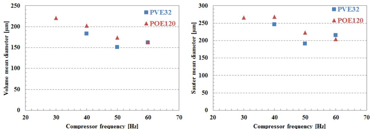
Figure 11: Volume mean diameter and Sauter mean diameter for the valve location
