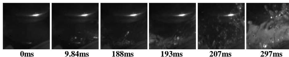
**Figure 3:** Startup sequence for compressor with PVE32 oil: initially oil droplets are generated by film breakup but afterwards liquid rushes in from the system due to high flow rate.
