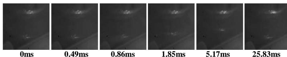
**Figure 4:** Opening sequence for discharge valve: note the cloud of small droplets that flows from the valve edge as the valve breaks open, very short period of time that cloud is noticeable.
