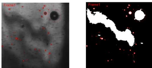
**Figure 6:** Raw and thresholded frame of a visualization movie: the red circles represent identified droplets, some are clearly not identified since they are out of the focal plane.
