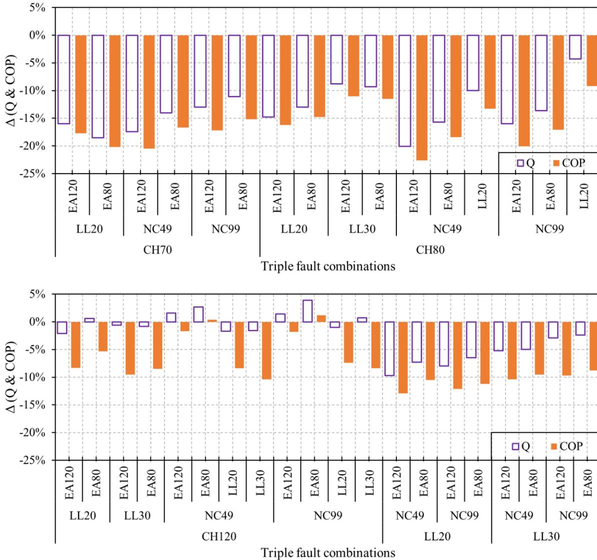
Figure 4: Triple fault impacts on cooling capacity and COP between two systems
