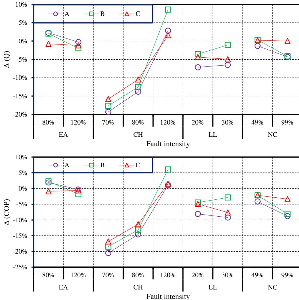
**Figure 2:** Single fault impacts on cooling capacity and COP between two systems
