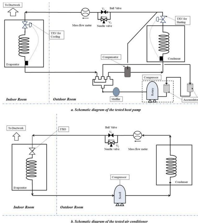
**Figure 1:** Schematic diagram of the tested systems (Hu and Yuill, 2021, 2022a)
