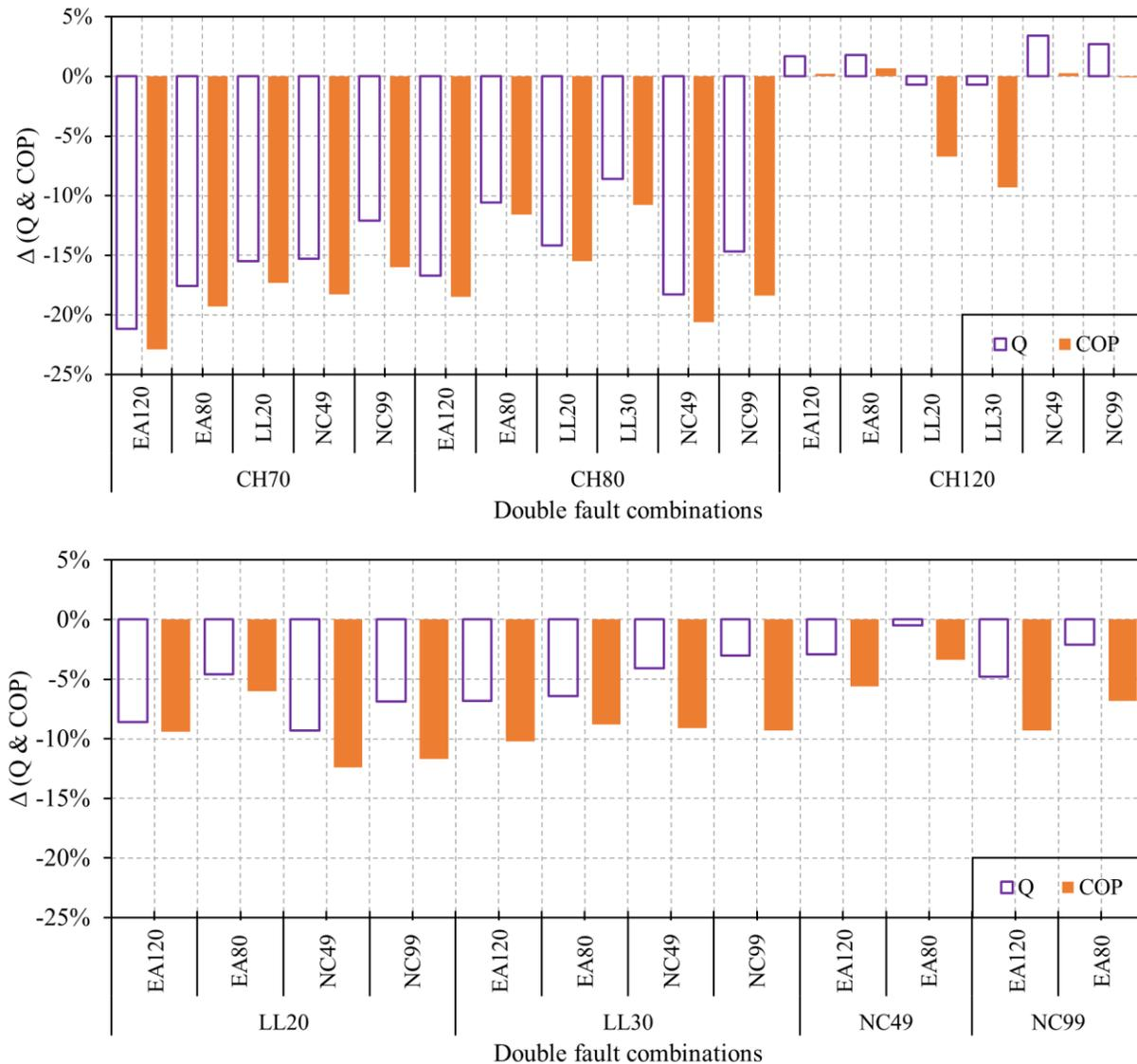
**Figure 3:** Double fault impacts on cooling capacity and COP between two systems
