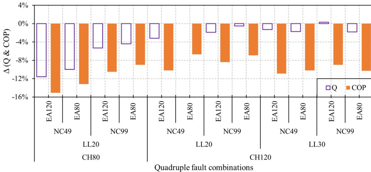
**Figure 5:** Quadruple fault impacts on cooling capacity and COP between two systems
