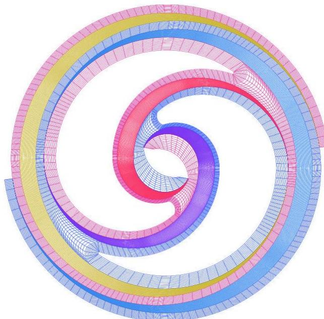
**Figure 5:** Numerical meshes of the working chambers and scroll vanes
