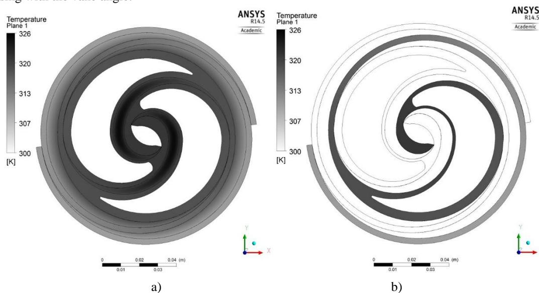
**Figure 6:** Temperature distribution without heat removal system
