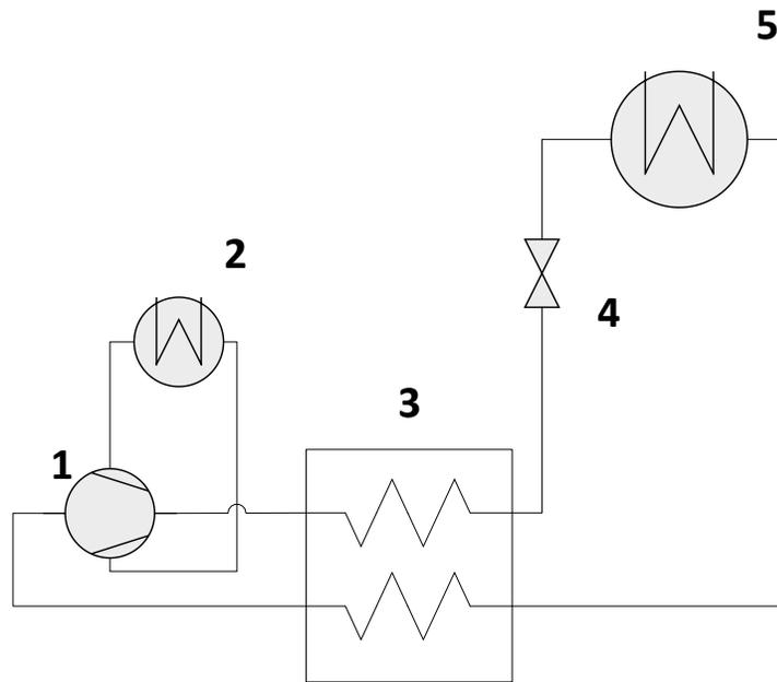
**Figure 4:** Joule-Thompson cryocooler cycle. 1) scroll compressor, 2) scroll cooling system, 3) heat exchanger, 4) J-T expansion, 5) evaporator
