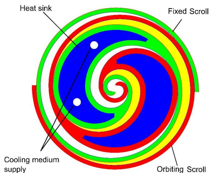
**Figure 1:** Hybrid vanes scroll compressor
