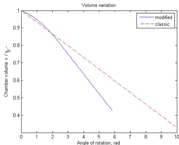
**Figure 3:** Volume change rate comparison for classical and modified vanes
