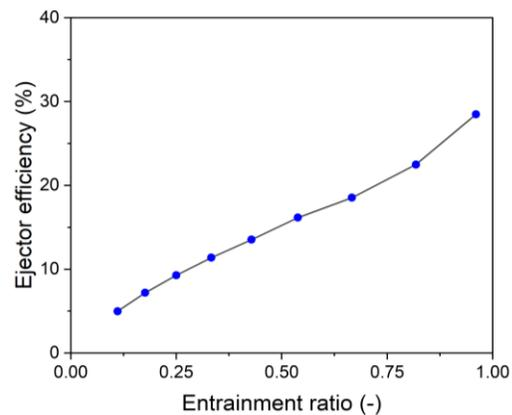
**Figure 5:** Variation of ejector efficiency with entrainment ratio
