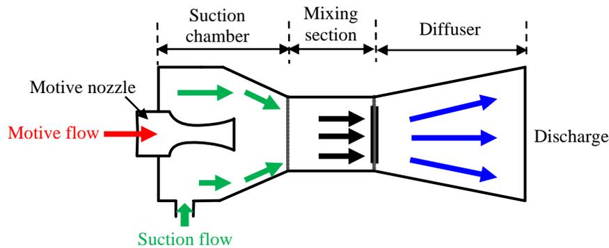
**Figure 1:** Schematic diagram of a two-phase ejector
