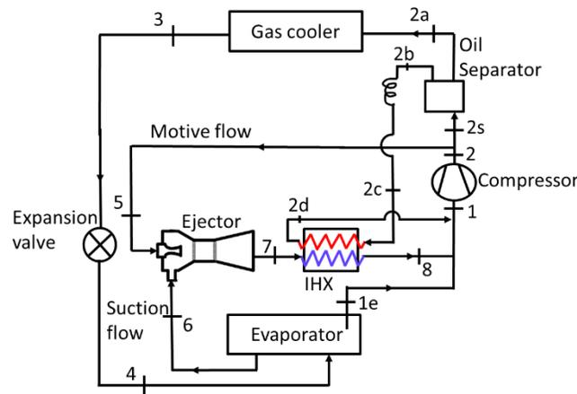
**Figure 2:** Schematic diagram of the ejector cycle patented by Kim *et al.* (2016)
