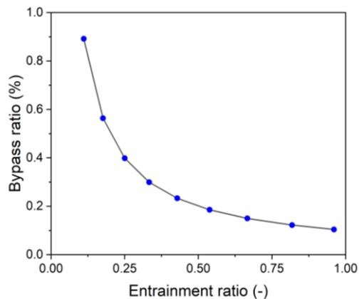
**Figure 4:** Variation of bypass ratio with entrainment ratio
