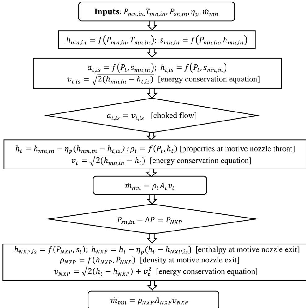
**Figure 6:** Design procedures of the motive nozzle for the ejector dedicated to oil pumping
