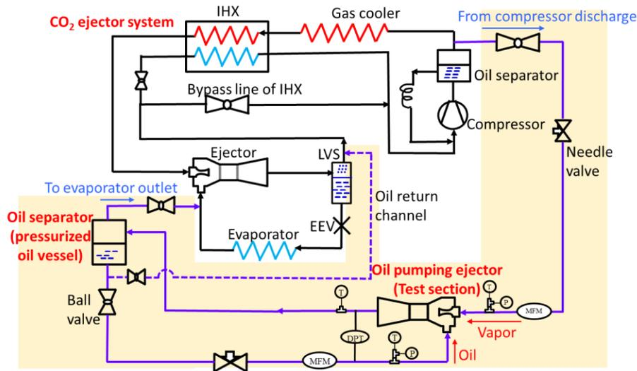
**Figure 7:** Test experimental layout design for oil entrainment experiments
