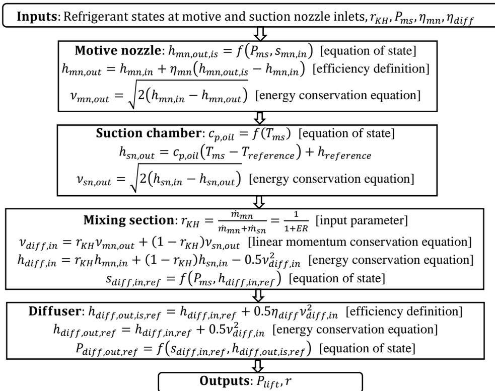
Figure 3: Ejector modeling procedure for the ejector cycle of oil pumping
