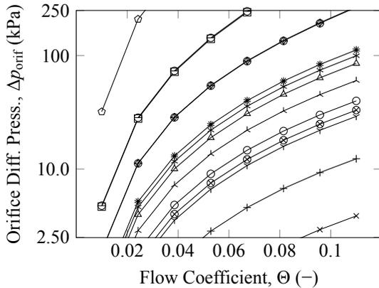
**Figure 5: Typical orifice selection results. The axis limits correspond to the acceptable measurement range, 10–990 inH<sub>2</sub>O.**
