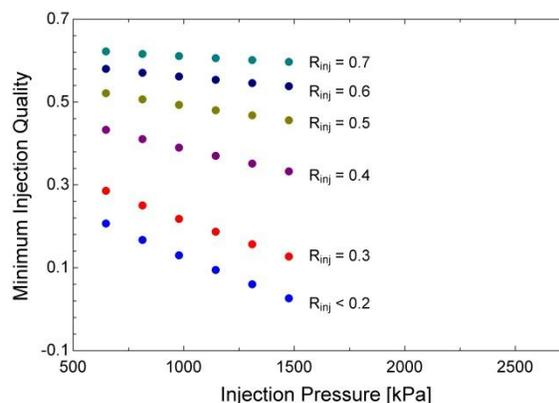
**Figure 6:** Minimum quality versus injection pressure (640 kPa suction pressure with 11°C superheat, 2290 kPa discharge pressure, and 24°C condensing temperature with 0°C subcooling)
