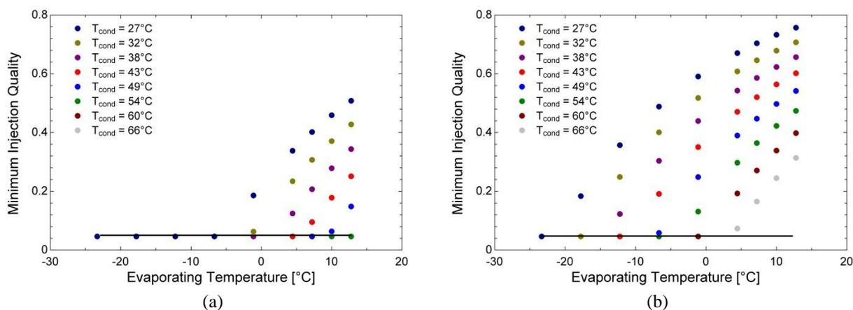
**Figure 3:** The dependence of minimum quality on inlet conditions when refrigerant is injected at 1000 kPa with a mass flow rate ratio of: (a) 0.2; (b) 0.4
