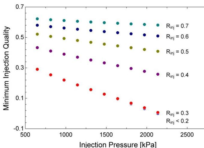
**Figure 4:** Minimum quality versus injection pressure (640 kPa suction pressure with 11 °C superheat, 2290 kPa discharge pressure, and 35 °C condensing temperature with 0 °C subcooling)
