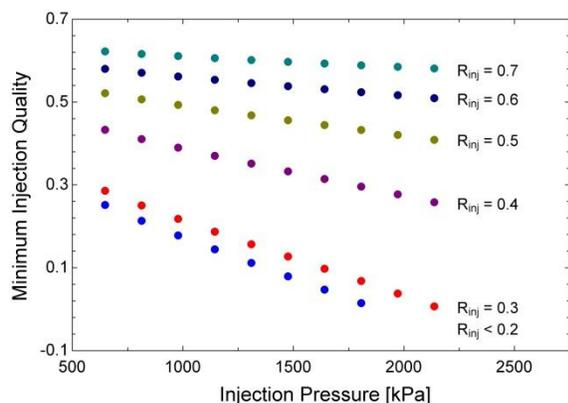
**Figure 5:** Minimum quality versus injection pressure (640 kPa suction pressure with 11°C superheat, 2290 kPa discharge pressure, and 35°C condensing temperature with 5°C subcooling)
