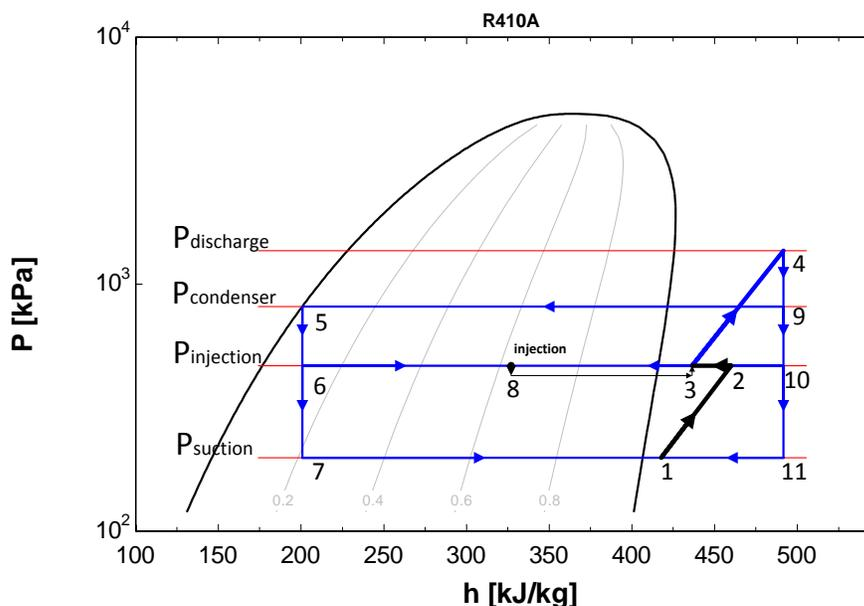
**Figure 2:** P-h diagram of load stand model with one injection port
