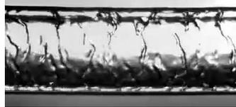
**Figure 8:** Annular mist flow at high OCR
