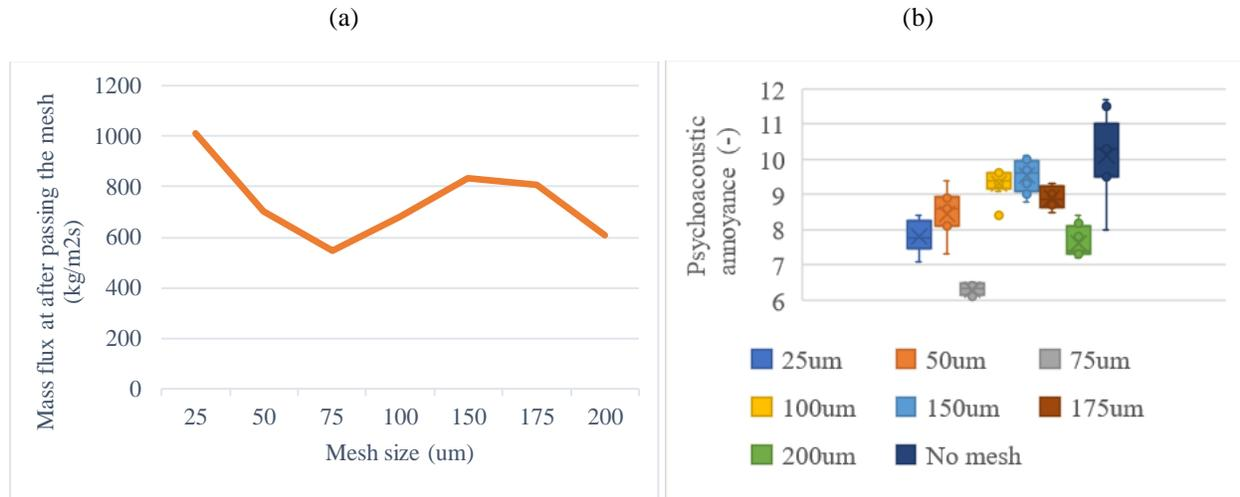
Figure 6. Noise mitigation effect for mesh with different sizes (a) relationship between the mesh size and mass flux after passing through the mesh (b) relationship between the mesh size and the psychoacoustic annoyance
