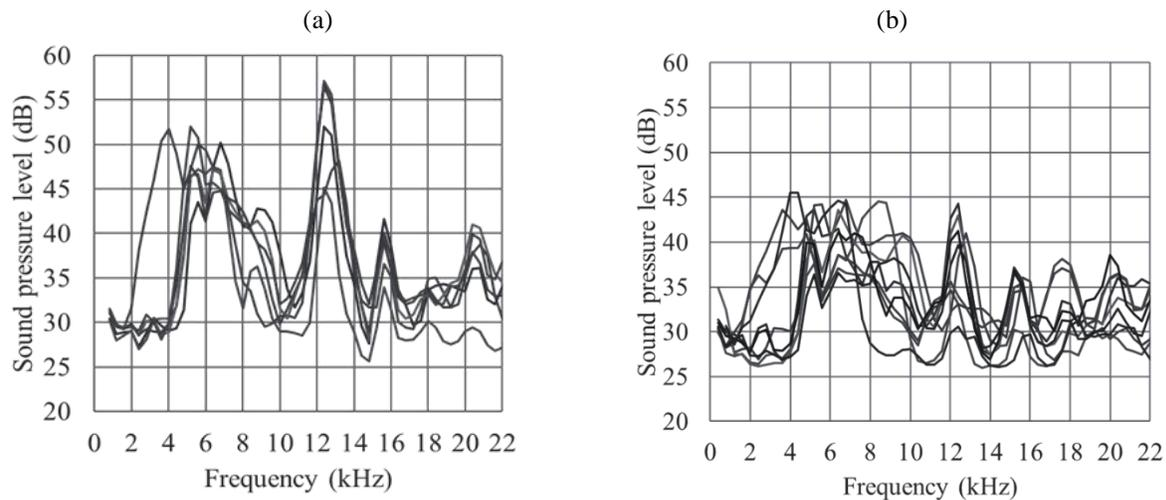
Figure 3. Spectra comparison of flow-induced noise for angle needle valve (a) without stainless steel mesh (b) with stainless steel mesh at the valve outlet
