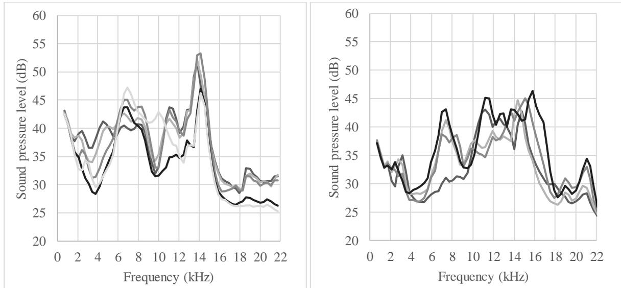
Figure 4. Spectra comparison of flow-induced noise near straight needle valve (a) without stainless steel mesh (b) with stainless steel mesh at the valve outlet
