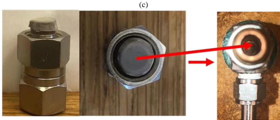
Figure 1. The installation of stainless-steel mesh (a) structure of stainless-steel mesh with 25um mesh size (b) type of expansion valves (c) position of mesh installation
