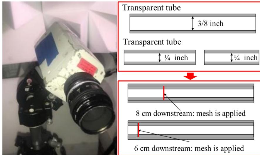
Figure 2. System schematic (a) experimental setup (b) high-speed camera (c) installation of mesh in the transparent tube
