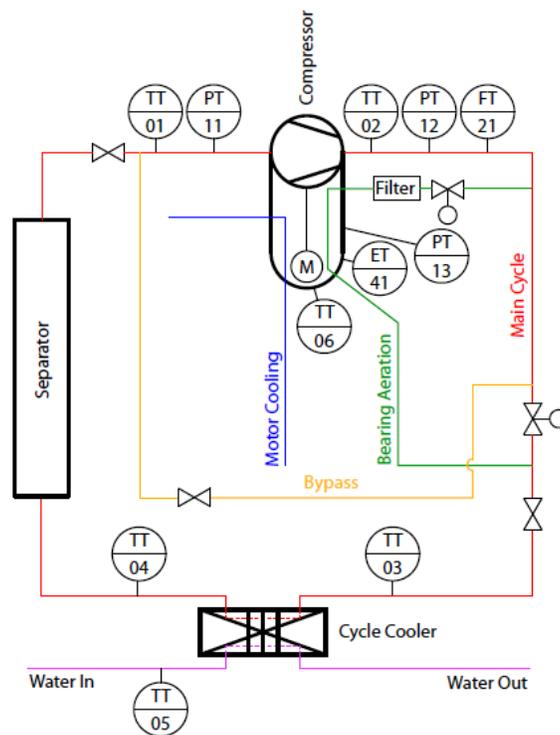
**Figure 5:** Representation of the vapor phase compressor test-rig indicating the main components and temperature (TT), pressure (PT), electrical power (EP), mass flow (FT) measurement locations. Further probes not indicated measure rotor speed and orbits.
