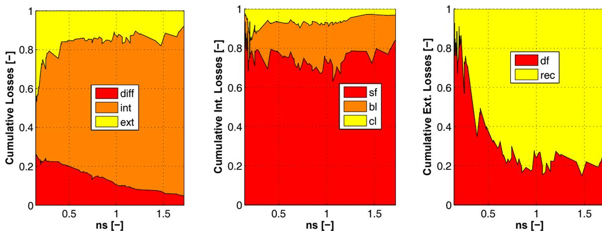
**Figure 9:** Split between (a) internal external and diffuser losses, (b) within the internal losses (sf: skin friction, bl: blade loading, cl: tip clearance losses, and (c) within the external losses (df: disc friction, rec: tip recirculation losses) as a function of the specific speed  $ns$ .
