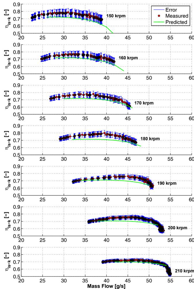
**Figure 7:** Measured and predicted internal isentropic efficiencies corresponding to the compressor map in Figure 6 for inlet conditions equivalent to an external air temperature of  $-12^{\circ}\text{C}$ .
