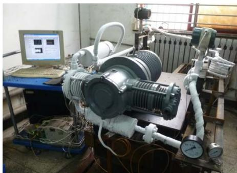
**Figure7:** Running experimental compressor and test rig
